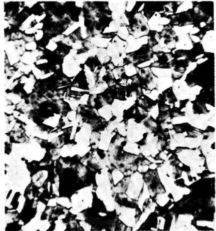
FIG. 6 — COPPER SHEET, ELECTROLYTICALLY POLISHED IN CHROMIC ACID SOLUTION (200 GM./L.). [Current density, 2 amp./sq. cm.; initial finish, "OOO"; etched in ammonium persulphate solution; \times 250 .]
