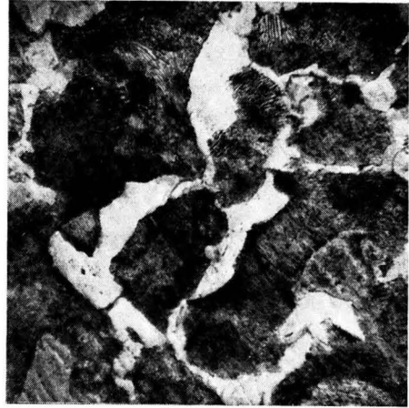
FIG. 2 — PLAIN CARBON HYPOEUTECTOID STEEL. [ Electrolyte : 50 per cent nitric acid + 50 per cent glacial acetic acid ; current density, 2 to 3 amp./sq. cm. ; initial finish, " OOO " ; time taken, 20 sec. ; etched in 2 per cent nital ; \times 900. ]
