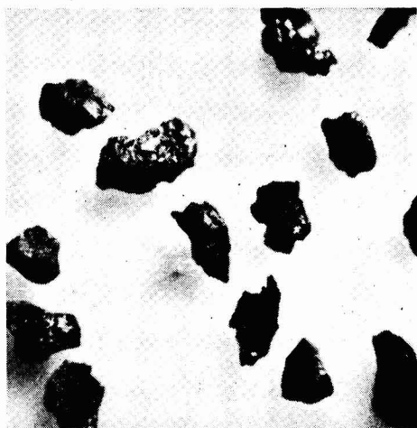
FIG. 8 — RETORT CARBON ( -40+50 MESH I.M.M.)
