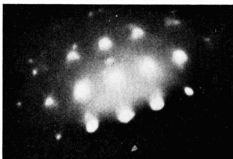
FIG. 4 — ELECTRON DIFFRACTION PATTERN OF SILVER FILM ON ROCK SALT CLEAVAGE FACE; BEAM ALONG [001] DIRECTION
