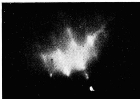
FIG. 2 — ELECTRON DIFFRACTION PATTERN OF ROCK SALT CLEAVAGE (100) FACE; BEAM ALONG [001] DIRECTION
