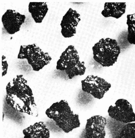
FIG. 7 — PETROLEUM COKE ( -30+40 MESH I.M.M.)
