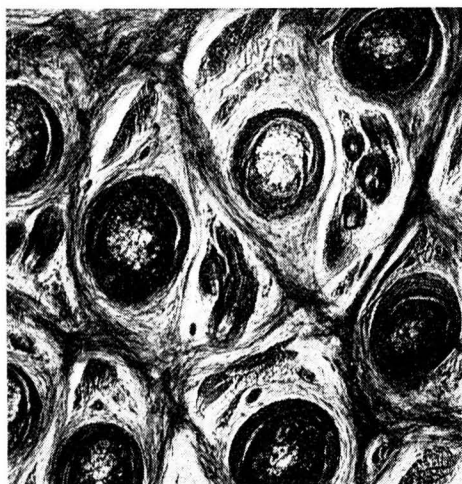
FIG. 4 — HORIZONTAL SECTION OF RED HAIRY SHEEP SKIN (THROUGH GRAIN LAYER) SHOWING ELASTIN NETWORK OF THE GRAIN ( \times 98 )
