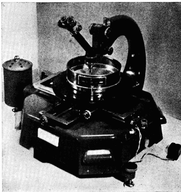
FIG. 1 — MICROMETER PROJECTOR FOR TESTING STANDARD SIEVES
