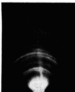
FIG. 2—ELECTRON DIFFRACTION PATTERN OF UNIDIRECTIONALLY RUBBED ONE-DEGREE ORIENTATED CuO; BEAM NORMAL TO THE RUBBING DIRECTION
