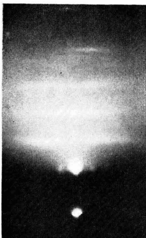
FIG. 1 — ELECTRON DIFFRACTION PATTERN OF A MONOMOLECULAR LAYER OF PARAFFIN WAX ON A SALT CRYSTAL [pattern shows that the surface is covered with a coherent layer of straight long-chain hydrocarbon molecules, closely packed together and standing vertically upright on the salt crystal surface]
