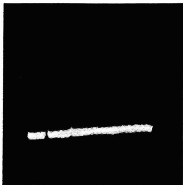
FIG. 9 — IONOSPHERIC REFLECTIONS ( F_2 REGION) OBTAINED WITH THE EQUIPMENT
