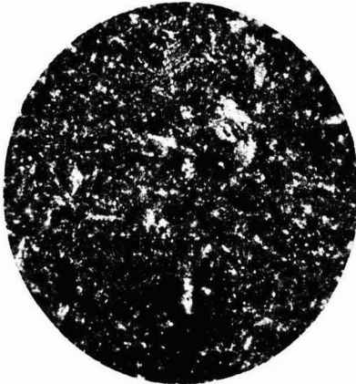
FIG. 7 — PHOTOMICROGRAPH OF 70 PER CENT \text{Al}_2\text{O}_3 COMPOSITION FIRED AT 1550^\circ\text{C} . \times 30 (CROSSED NICOLS) SHOWING MOSTLY MULLITE WITH SOME CORUNDUM
