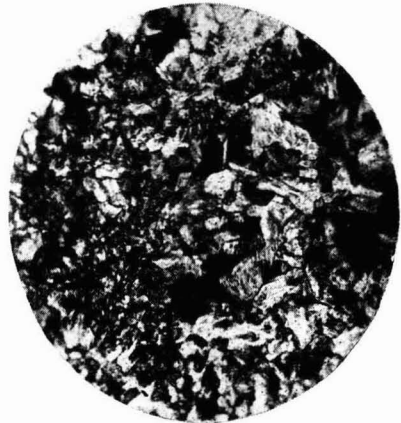
FIG. 4 — PHOTOMICROGRAPH OF SHEVAROY WHITE BAUXITE \times 30 [Bauxite grains are seen with specks of Fe_2O_3 ]
