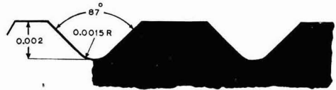
FIG. 4 — SHAPE OF THE GROOVE MADE ON THE RECORD
