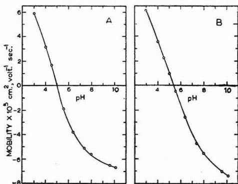
Fig. 3—pH-mobility curve of (A) fraction obtained by 70 per cent ammonium sulphate saturation at ionic strength 0.1 and (B) fraction III obtained by combined sodium and ammonium sulphate fractionation at ionic strength 0.1
