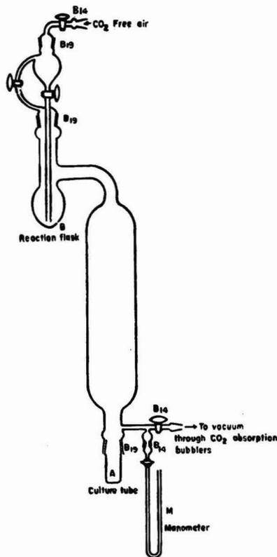
Fig. 1 — Apparatus for the fixation of carbon dioxide
