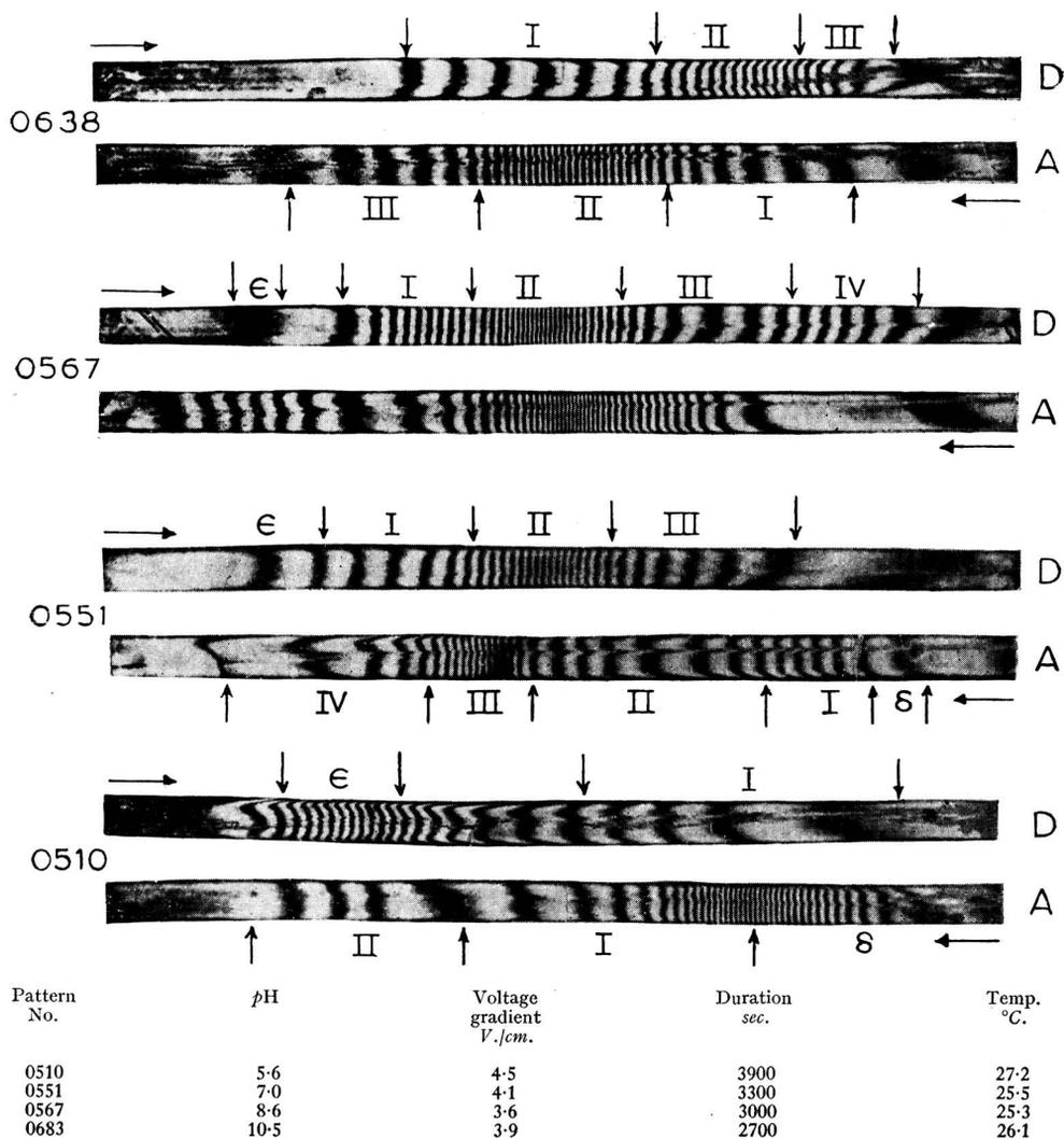
Fig. 1 — Typical electrophoretic patterns of black gram meal proteins at various pH values and ionic strength 0.1 [A, ascending pattern; D, descending pattern; I, II, III and IV are components]
