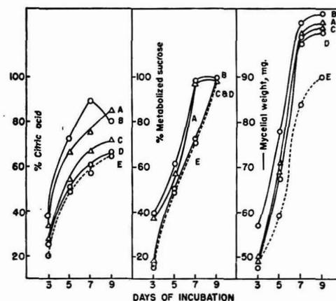
Fig. 4 — Citric acid production under excess CO<sub>2</sub> tension (commercial cane sugar as C source) [(A) 0.1 per cent CO<sub>2</sub>, (B) 0.5 per cent CO<sub>2</sub>, (C) 1.0 per cent CO<sub>2</sub>, (D) 2.0 per cent CO<sub>2</sub> and (E) control]
