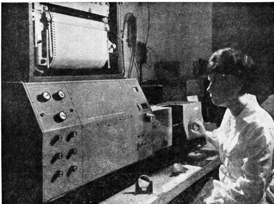
Unicam SP700C as used for characterisation of visible and infrared filters at Standard Telephones & Cables Ltd. (Rectifier Division), Harlow, Essex (By kind permission of Standard Telephones & Cables Ltd. Rectifier Division Harlow, Essex)
