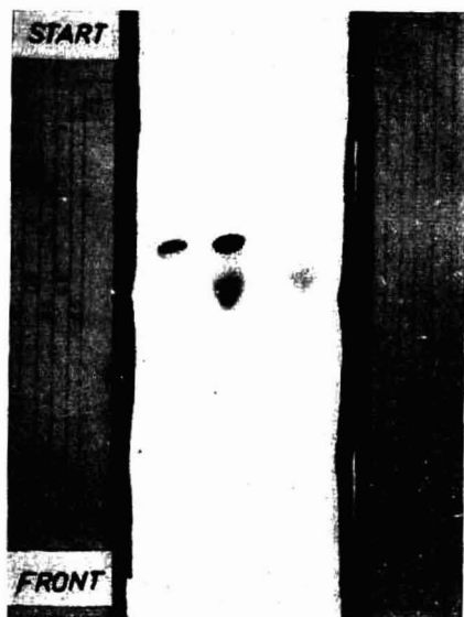
Fig. 1. Chromatogram of a simple mixture of 2,4-dinitrophenylhydrazones. From left to right: formaldehyde, formaldehyde + methyl ethyl ketone (mixture); methyl ethyl ketone.
