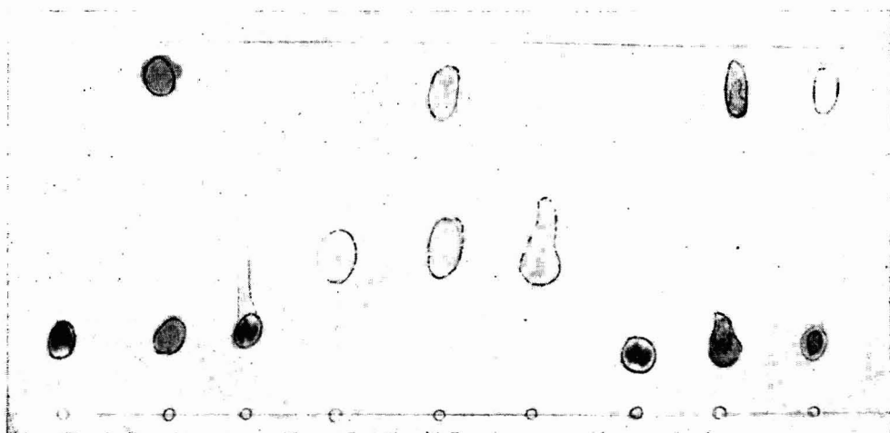
Fig. 1. Chromatogram of some dyestuffs mixed with cetyltrimethylammonium bromide. Solvent: butanol-acetic acid-water (100:20:80). From left to right: Scharlach GN; Scharlach GN mixed with a 10% solution of cetyltrimethylammonium bromide; Scharlach GN mixed with a 1% solution of cetyltrimethylammonium bromide; C.I. Acid Blue 3 alone and mixed with 10% and 1% cetyltrimethylammonium bromide. Bottom line: line of application of spots. Top line: liquid front.
