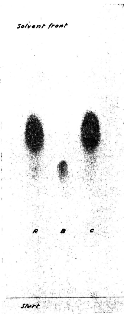
Fig. 3. Thin-layer chromatography on Silicagel "G". 15 cm run; solvent No. 1. A = tablet containing 14% beef extract + 1% whale extract; B = 3-methylhistidine; C = tablet containing 15% beef extract.
