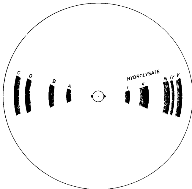
Fig. 1. Circular paper chromatography of soybean-sapogenols A, B, C, D and of the acid hydrolysate of soybean saponins. Paper: Whatman No. 3MM. Solvent: hexane-chloroform-acetic acid (100:10:2.5). Developing reagent: \text{SbCl}_3 in chloroform.
