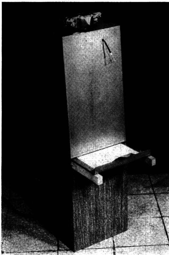
Fig. 5. Apparatus for detection by photography of the chromatograms in U.V. light. Distances: camera-chromatogram, 45 cm; chromatogram-U.V. lamp, 35 cm.
