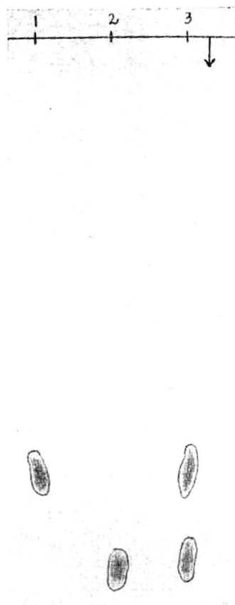
Fig. 1. Paper chromatographic separation of glucuronic and galacturonic acids. Solvent: acetone-ethanol-isopropyl alcohol-borate buffer, pH 10.0 (3:1:1:2). 1 = galacturonic acid; 2 = glucuronic acid; 3 = mixture.
