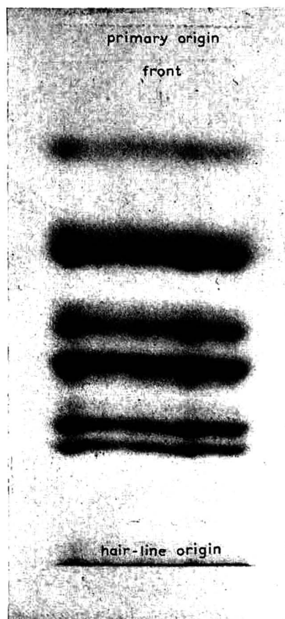
Fig. 2. One-dimensional continuous development of Oil Red OS from a hair-line origin. Adsorbent: silicagel G. Solvent: carbon tetrachloride. Time: 18 h. Distance from origin to front: 15 cm.
