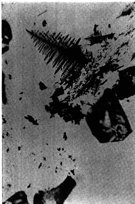
Fig. 9. Carbazole crystal transferred among the silica gel grains (the approximate diameter of a grain is 0.15 mm).
