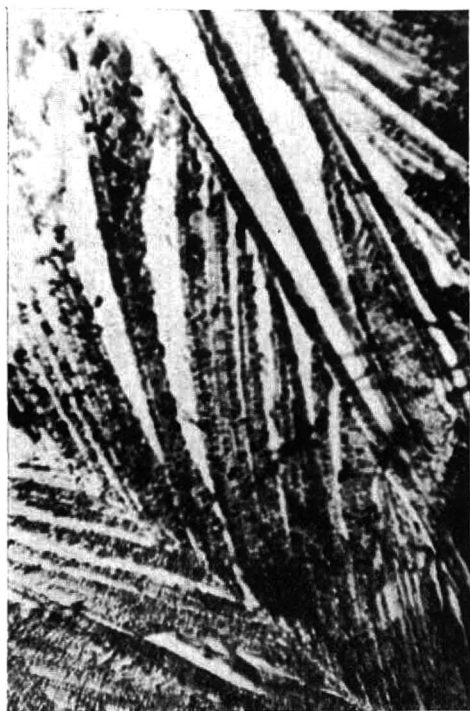
Fig. 2. Start line of the acenaphthene zone (magnified 50\times ).
