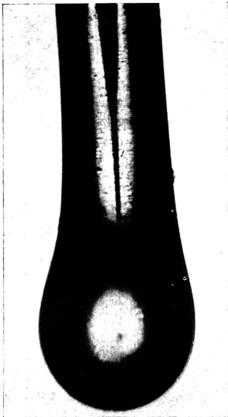
Fig. 7. Glass rod with ball for the transfer of microcrystals (thickness of the rod 0.10 mm, ball diameter 0.15 mm).
