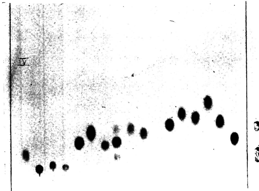
Fig. 2. A single 15 cm development in the formic acid-methyl ethyl ketone- tert. -butanol-water solvent. The sugars are in the same sequence as in Fig. 1.
