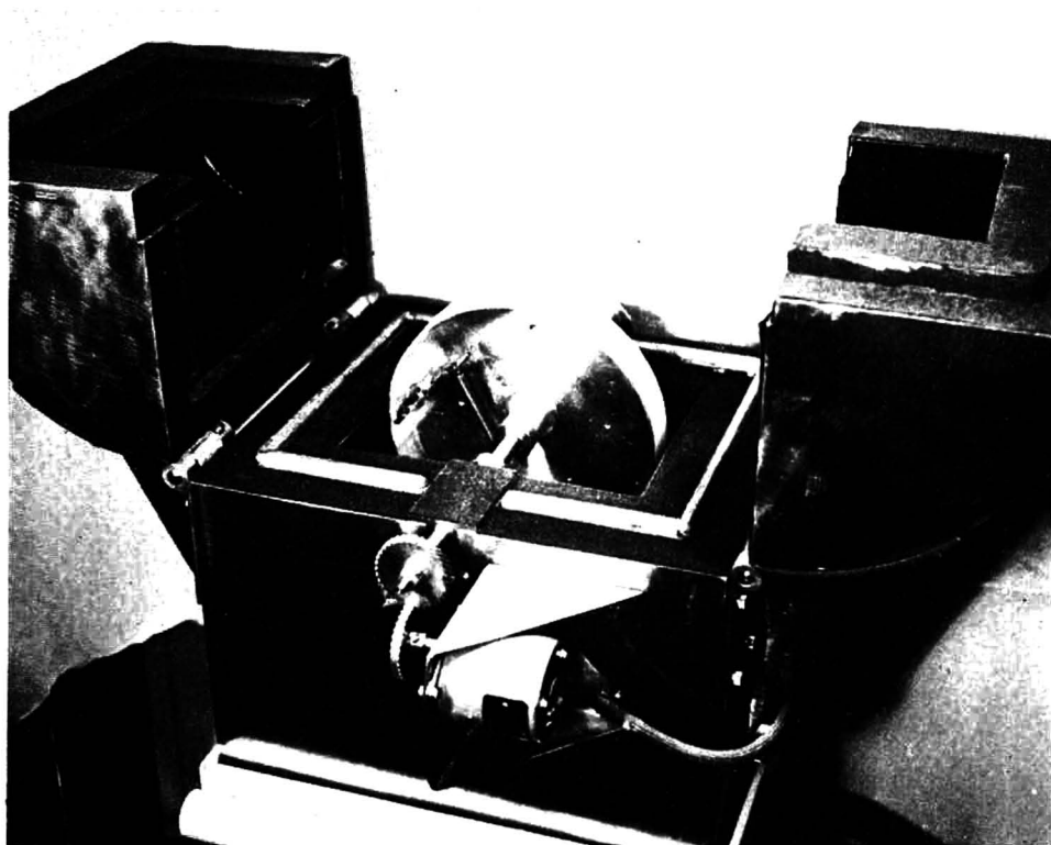
Fig. 2. View of instrument with open lids to show mounting of chromatograms.
