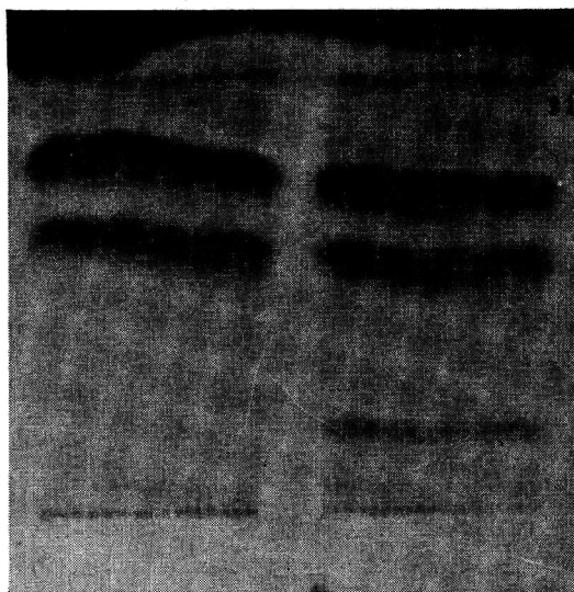
Fig. 3. Chromatogram with solvent 2, continuous development for 3 h. Left: oil 25 mg; right: progesterone 250 \mu g in 25 mg oil. From bottom to top: progesterone clearly separated from the two diglyceride bands. Detection: iodine vapor.
