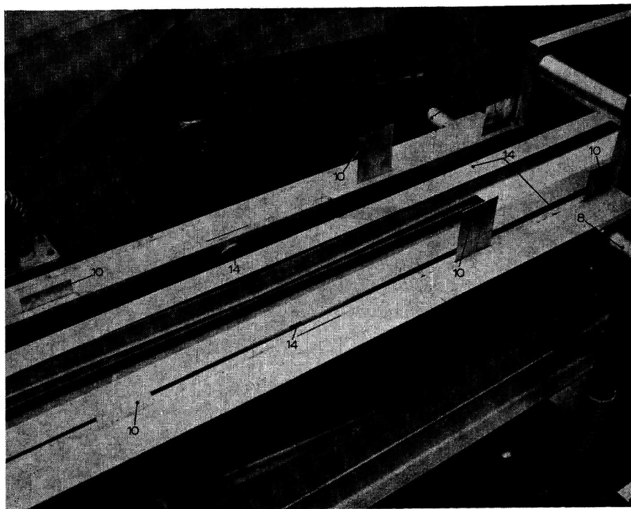
Fig. 4. The reaction-chamber with lid removed to show arrangement of the belting system. A strip of paper is entering from the right. The central guideposts (14) are visible: the first pair are not visible but their position is indicated by the reference numbers. (Other reference numbers as in Fig. 2a.) The upper and lower belts are seen on their return passage through the reaction chamber.
