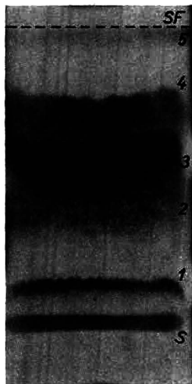
Fig. 2. Preparative chromatography of crude DNP-derivatives on Whatman No. 3 silica gel paper impregnated with sodium tetraborate in chloroform-methanol (100:0.5). Detection: U.V. light (254 nm). DNP-derivatives: 1 = phytosphingosines; 2 = threo-sphingosines; 3 = erythro-sphingosines; 4 = dihydro-sphingosines + unidentified degradation products I; 5 = O-methyl-derivatives + unidentified degradation products II + 2,4-dinitrophenol; S = start; SF = solvent front.
