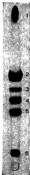
Fig. 1. Separation of dehydrated alfalfa xanthophylls and carotene by TLC. 1 = \beta -Carotene; 2 = lutein; 3 = xanthophyll No. 2; 4 = violaxanthin; 5 = xanthophyll No. 1; 6 = neoxanthin.
