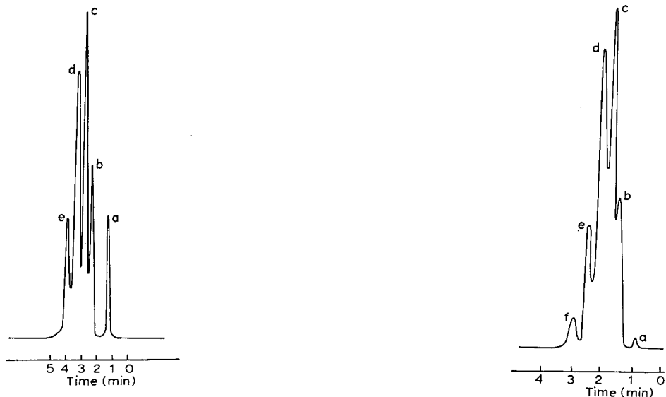
Fig. 1. Experiment A2. Reaction between O = P(OMe)_3 and O = P(OEt)_3 . (a) = Diethyl ether, (b) = O = P(OMe)_3 , (c) = O = P(OMe)_2(OEt) , (d) = O = P(OMe)(OEt)_2 , (e) = O = P(OEt)_3 .
