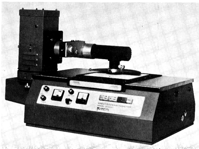
Fig. 1. The densitometer (Schoeffel Instr. Co., Westwood, N.J., U.S.A.). Model SD 3000 (about \frac{1}{10} of original size).
