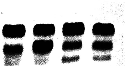
Fig. 1. Thin-layer gel filtration of serum proteins on Sephadex G-200. Sample: 10 \mu l of undiluted serum proteins. Plate 20 \times 20 cm. Separation time: 6 h. Staining with Amido Black 10B. From left to right: human, horse, pig and bovine serum. From top to bottom: 4s, 7s and 19s components of serum.
