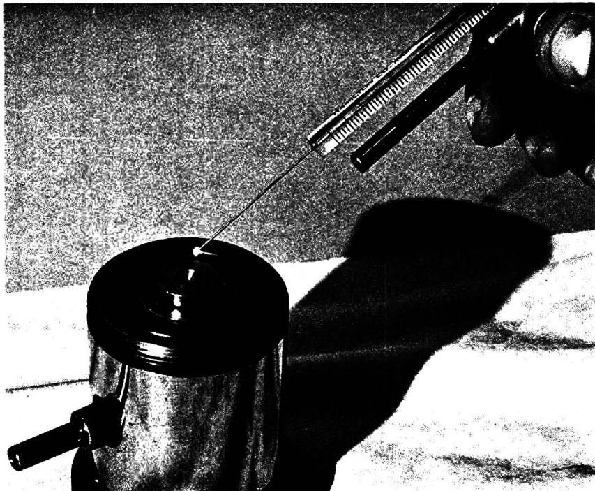
Fig. 2. Syringe technique for transferring microgram components to KBr powder.
