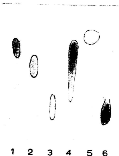
Fig. 2. Thin-layer gel filtration on agar of the MBS fractions from column gel filtration. Pearl-condensed agar, 4%, particle size 100–400 mesh. Plates 8 \times 14 cm; thickness of the layers 0.4 mm; buffer 0.1 M Tris + 0.1 M NaCl + HCl, pH 7; flow rate 1.5 cm/h; 20 \mu l of 0.5–2% protein solution applied. 1, 2, 3 = fractions from Fig. 1, 4 = unfractionated MBS; 5 = Bromphenol Blue; 6 = dilution of Indian ink.
