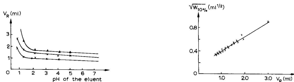
Fig. 1. Dependence of the retention volumes on the pH of the 0.05 M Na 2 SO 4 eluent. Column: 1 m long packed with Zipax SCX, thermostatted to 30.0°, flow-rate 0.40 ml/min.
