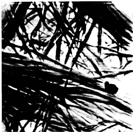
Fig. 7. Electron micrograph of a sample of fibrous cerium(IV) phosphate (magnification 10,000 \times ).
