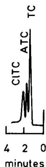
Fig. 1. Separation of TC, ATC and CITC on Perkin-Elmer Sil-X ( 13\ \mu\text{m} ). Column, 5 \times 125\ \text{mm} . Eluent, ( 0.1\ \text{M}\ \text{HClO}_4 + 1.9\ \text{M}\ \text{NaClO}_4 + 0.005\ \text{M} citric acid)-acetonitrile (2:1) (v/v). Eluent velocity, 2.6 mm/sec. Detector, UV photometer, wavelength 280 nm, sensitivity 0.2 absorbance units full scale deflection (a.u.f.s.). Sample about 100 ng of each component.
