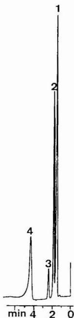
Fig. 7. Chromatogram of tooth-paste extract (conditions as in Fig. 1). Peaks: 1 = water; 2 = ethylene glycol; 3 = glycerol; 4 = xylitol.
