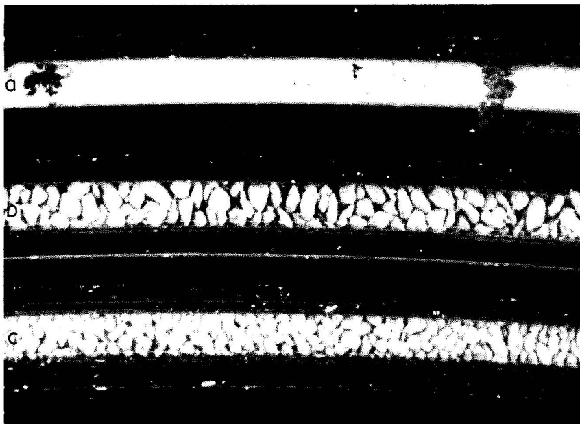
Fig. 1. Microphotographs of 0.45-mm I.D. columns filled with GTCB Sterling MT (Phase Separations, Solingen, G.F.R.). (a) PLOT column; (b) and (c) micro-packed columns with particle sizes of 0.16–0.20 and 0.09–0.12 mm, respectively.
