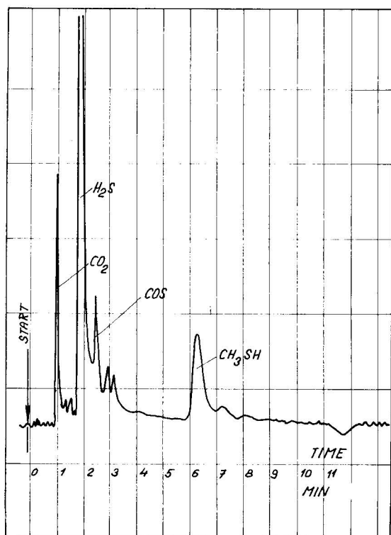
Fig. 4. Chromatogram of waste gas. Injection of 0.2 ml. Conditions as in Fig. 3 and Table I.
