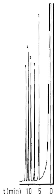
Fig. 3. Gas chromatogram of silylated triazines. 4 \cdot 10^{-11} A.f.s.d.; 0.5 \mu l injected; 140–200° at 4°/min; each peak represents 25 ng. Peaks: 1 = CA (164°); 2 = Ad (172°); 3 = An (179°); 4 = Mn (184°); 5 = Ph (192°).
