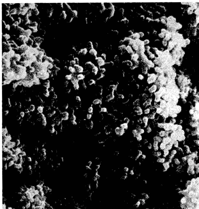
Fig. 19. SEM of whisker formation on the inner surface of soft glass produced by etching with HF. Reprinted with permission 151 .
