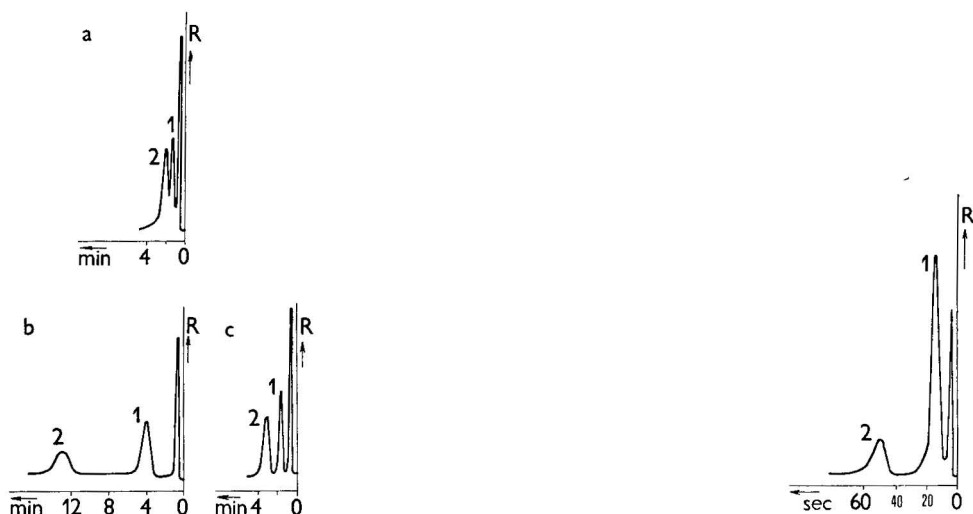
Fig. 4. Separation of a mixture of aromatic amines: 1 = aniline; 2 = N,N-dimethylaniline. Micro-packed columns ( 295 \times 1 mm I.D.). (a) Porasil C, 220^\circ , u = 20.3 mm/sec; (b) Porasil C modified with phthalocyanine, 220^\circ ; (c) Porasil C modified with phthalocyanine, 250^\circ .
