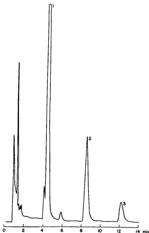
Fig. 1. Gas chromatogram of rainbow trout exposed to 15 ppm aminocarb for 144 h. Peaks: 1 = aminocarb; 2 = AM; 3 = MA.
