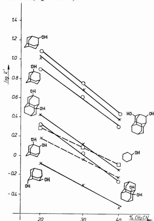
Fig. 3. Variation of the  $\log k'$  with the concentration of acetonitrile in the mobile phase (water-acetonitrile).
