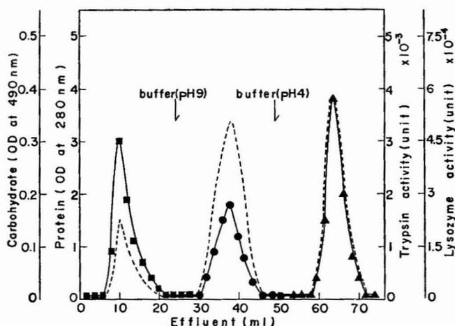
Fig. 5. Separation of a mixture of trypsin, lysozyme and ovalbumin on immobilized tannin. Two millilitres of protein solution (pH 7.5) containing 10 mg of trypsin, 10 mg of ovalbumin and 10 mg of lysozyme were applied to the column, and the proteins adsorbed were eluted with the specified buffer solutions. Other conditions are given in the text. ■—■, Trypsin activity; ●—●, carbohydrate; ▲—▲, lysozyme activity; ---, protein.
