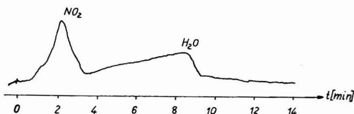
Fig. 5. Analysis of  $\text{NO}_2$  in a glass blower's workshop. Column:  $1 \text{ m} \times 4 \text{ mm}$  I.D., PTFE, 10% Fluorolube-oil on Fluoropak 80. Temperature:  $30^\circ\text{C}$ . Concentration of amine: 100 ppm. Sample size:  $\text{NO}_2$  enriched from 130 ml.  $\text{NO}_2$  room concentration: 1 ppm.
