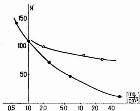
Fig. 6. Chromatography of L-leucine showing the number of effective plates per 10 cm of column length,  $N'$ , as a function of the amount of L-Leu per  $\text{cm}^2$  of the column cross-section.  $\circ$ — $\circ$ , Column  $340 \times 10$  mm; eluent  $0.2 N \text{NH}_4\text{OH}$ , flow-rate 60 ml/h.  $\bullet$ — $\bullet$ , Column  $140 \times 9$  mm, flow-rate 50 ml/h.
