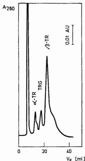
Fig. 4. Separation of components of crude trypsin and trypsinogen. Sample: 1.2 mg of commercial trypsin and 0.15 mg of trypsinogen in 70  $\mu$ l of the elution buffer. Flow-rate: 7 ml/h at 22°C. Other conditions as in Fig. 1.2. TRG = Trypsinogen.
