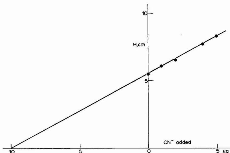
Fig. 3. Standard additions plot for the results in Table V.
