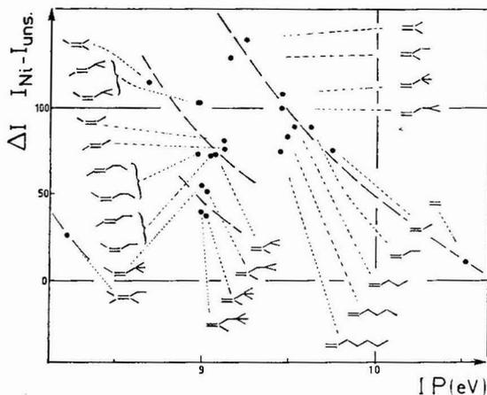
Fig. 10. Specific contribution to retention ( $\Delta I$ ) due to the nickel form of the ion exchanger relative to the unsulfonated copolymer matrix (uns.) as a function of ionization potential of the alkene (IP). Decrease of the specific interaction with degree of substitution, branchings or bulky groups for di- or tetrasubstituted ethylenes suggest a dominant influence of steric effects.
