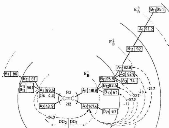
Fig. 9. Topological information diagram for retention of alkenes on the nickel form of the ion exchanger showing some interaction parameters. The negative contribution of these parameters to retention on the  $Ni^{2+}$  form underlines the sensitivity of the specific  $\pi$  double bond-Ni interactions to branchings and bulky groups in the homologous series of geminal 1-alkenes.
