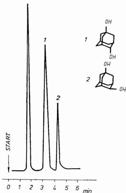
Fig. 2. Separation of the two adamantane-1,4-diol stereoisomers. Column, MicroPak CH-10; mobile phase, methanol-water (30:70); flow-rate, 10 ml/h; temperature, 30°C.
