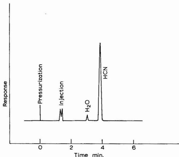
Fig. 1. Gas chromatogram obtained from a 0.10 ppm aqueous solution of cyanide.
