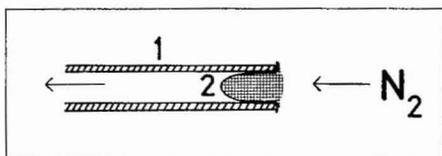
Fig. 1. Diagram showing sample application part placed inside the Pt-coil of the probe. 1 = Quartz tube; 2 = sample holder.
