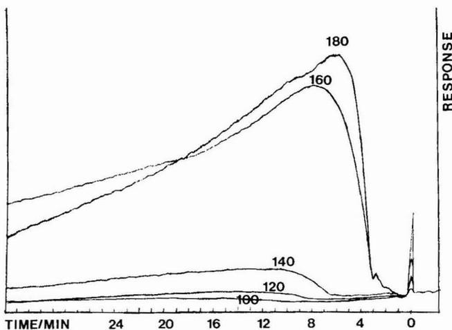
Fig. 5. Chromatogram from injections of  $2 \mu\text{l}$  of water at various temperatures ( $100\text{--}180^\circ\text{C}$ ) with FID. Attenuation:  $4 \cdot 10^{-11}$  A.f.s. Other conditions as in Fig. 1.
