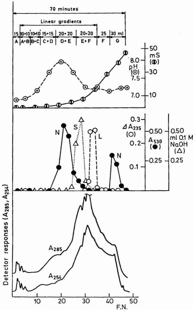
Fig. 7. Chromatography of 25 mg of Pectinex Ultra on Spheron DEAE-1000 with an adjusted gradient elution with buffers of pH 7. The buffers were prepared as in Fig. 5 and the labelling of enzymatic activities is also the same. Fractions 5.1 ml per 90 sec; pressure 0.6 MPa. F.N. = fraction number.
