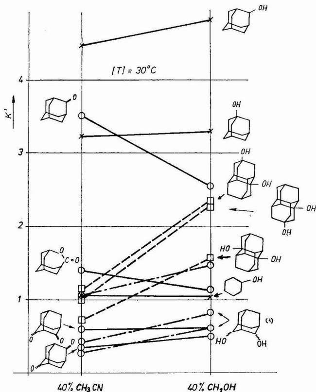
Fig. 6. Comparison of the capacity factors of some compounds, measured in two different mobile phases.
