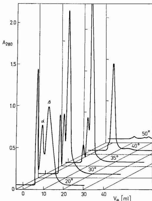
Fig. 3. Elution profiles of a commercial trypsin sample on HIC at different temperatures. The conditions are as in Fig. 1.1, except for temperature.
