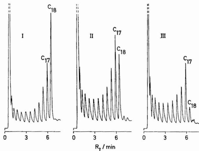
Fig. 4. Pyrograms of three different  $C_{18}$  materials. I = ODMCS-silica; II = OMDCS-silica; III = OTCS-silica. GC system B. For explanation see Table I.
