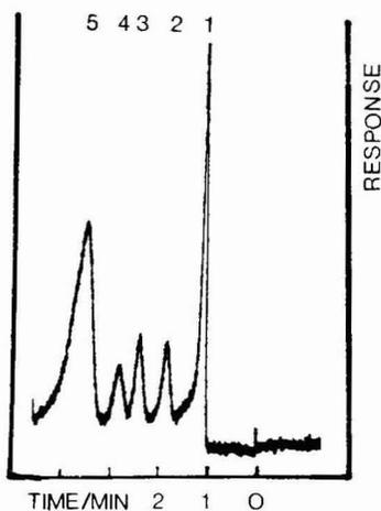
Fig. 3. Chromatogram of volatile amines in ethanol with 500 ppm ammonia added. Solute concentrations: 1–3, about 0.03 ppm; 4, about 0.15 ppm. Sample size 1.8  $\mu$ l. Solutes: 1 = ammonia; 2 = methylamine; 3 = dimethylamine; 4 = ethylamine; 5 = isopropylamine. Temperature: 5 min at 80°C, programmed from 80 to 120°C at 20°C/min, then 5 min at 120°C. Attenuation:  $1 \cdot 10^{-12}$  A.f.s. Other conditions as in Fig. 1.
