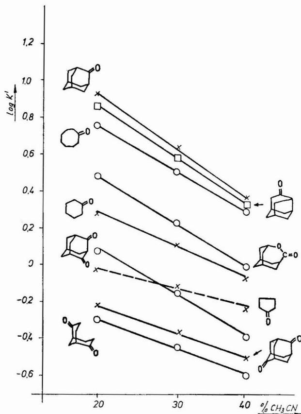
Fig. 4. Variation  $\log k'$  with the concentration of acetonitrile in the mobile phase (water-acetonitrile).
