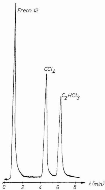
Fig. 3. Analysis of halocarbons in air. Column: 2 m × 4 mm I.D., glass, 10% SE-30 on Chromosorb W AW DMCS. Temperatures: column, 30°C; oven: 960°C. Sample size: 50  $\mu$ l with 100 ppm Freon 12, CCl<sub>4</sub> and C<sub>2</sub>HCl<sub>3</sub>.
