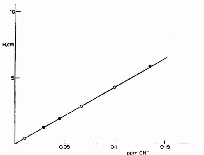
Fig. 2. Calibration graph obtained from standard aqueous solutions of (○) cyanide and (●) thiocyanate as cyanide.
