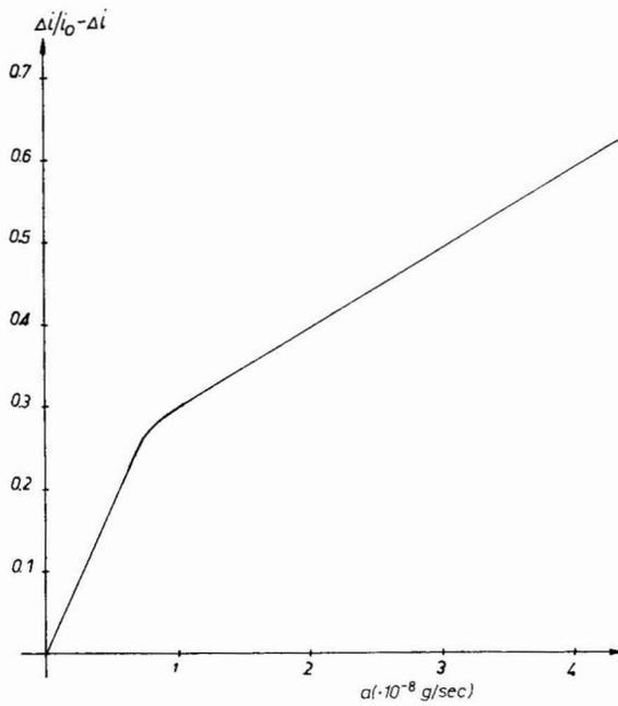
Fig. 2. Linearity of the AID. Sample: Freon 12.
