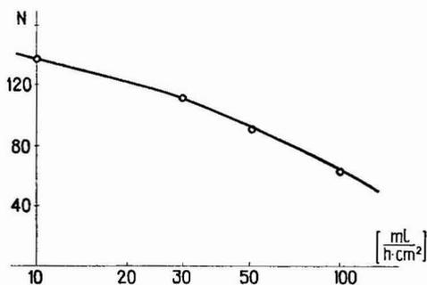
Fig. 5. Chromatography of 2.0 mg L-Leu showing the number of effective plates,  $N$ , as a function of elution rate. Column:  $140 \times 9$  mm.
