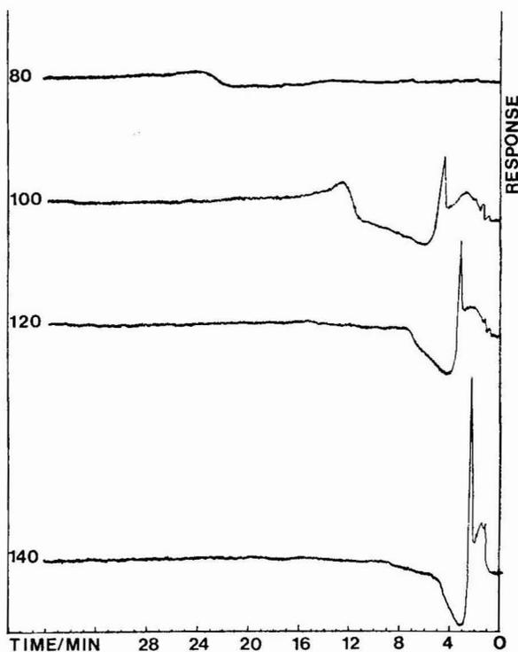
Fig. 4. Chromatograms from injections of  $2 \mu\text{l}$  of water at various temperatures ( $80\text{--}140^\circ\text{C}$ ) with TSD. Attenuation:  $1 \cdot 10^{-12}$  A.f.s. Other conditions as in Fig. 1.
