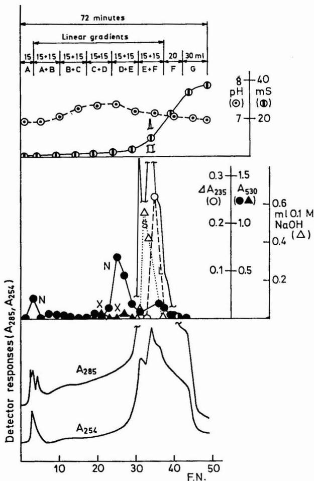
Fig. 5. Chromatography of 25 mg of Pectinex Ultra on the anion exchanger Spheron DEAE-1000, eluting with buffers of pH 7. Fractions 4.4 ml per 90 sec; pressure 0.4 MPa. The buffers were prepared from hydrochloric acid of the given concentration, which was adjusted with Tris to pH 7: A, 0.005 M; B, 0.05 M; C, 0.1 M; D, 0.2 M; E, 0.4 M; F, buffer E with 1 M sodium chloride; G, 0.2 M sodium chloride. Enzymatic activities as in Figs. 1 and 3. F.N. = fraction number.
