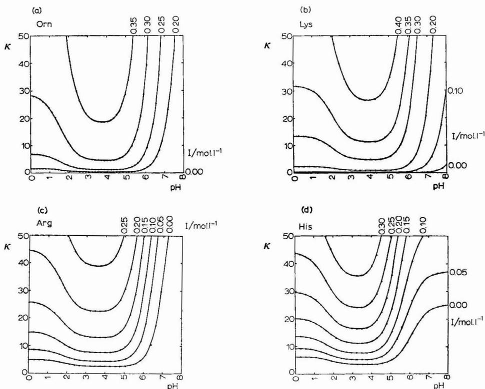
Fig. 1. The effect of the eluent pH on the capacity ratios of different ampholytes at the constant ionic strengths. (a) Ornithine; (b) lysine; (c) arginine; (d) histidine.
