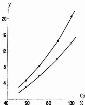
Fig. 1. Retention volumes of leucine enantiomers as a function of the degree of sorbent saturation by  $\text{Cu}^{2+}$ . ●—●,  $V_D$ ; ○—○,  $V_L$ . Column:  $140 \times 9$  mm. Eluent:  $0.2 N \text{NH}_4\text{OH}$ ; flow-rate 50 ml/h.
