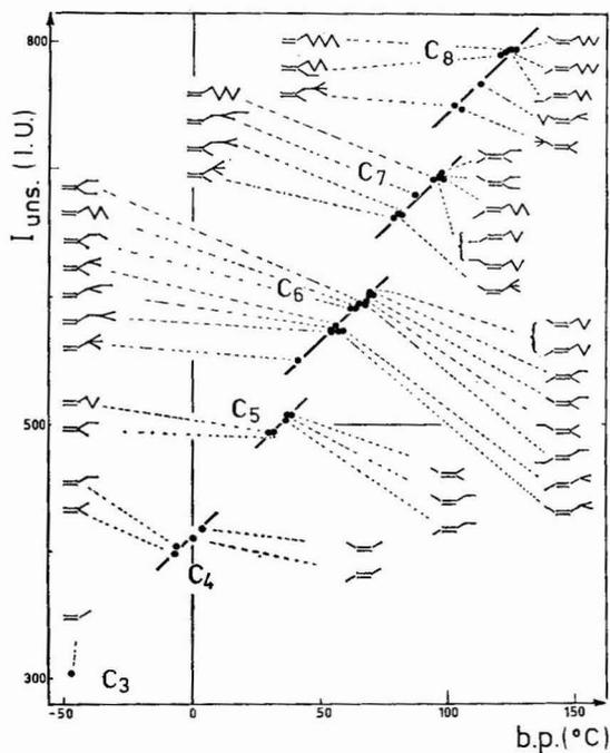
Fig. 6. Retention index of alkenes ( $I_{\text{uns}}$ ) on the unsulfonated copolymer, in index units (I.U.), as a function of boiling point of the alkene. Regular trends are observed for every subpopulation (from  $C_4$  up to  $C_8$ ).
