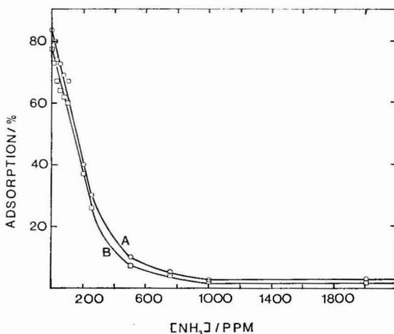
Fig. 7. Percentage adsorption of methylamine (A) and dimethylamine (B) at various concentrations of ammonia and with ethanol as solvent. Solute concentration 0.03 ppm. Column temperature 80°C. Attenuation:  $1 \cdot 10^{-12}$  A.f.s. Other conditions as in Fig. 1.
