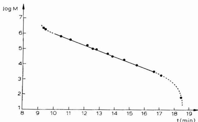
Fig. 2. Retention times vs. logarithm of the molecular weight of PS standards. Column ( $330 \times 0.6$  mm) packed with a mixture of LiChrospher Si 100 and Si 1000 sorbents. Eluent: methylene chloride; flow-rate  $4.6 \mu\text{l}/\text{min}$ . Sample volume:  $0.3 \mu\text{l}$  ( $1 \text{ mg}/\text{ml}$ ).
