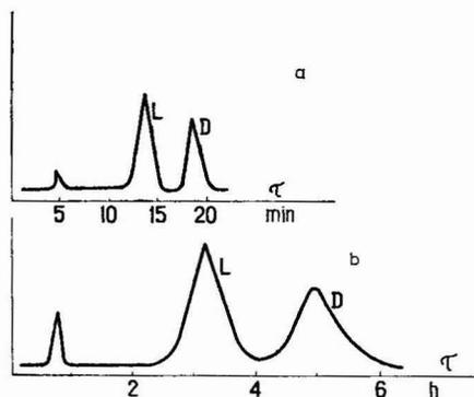
Fig. 7. Chromatography of L,D-leucine on a sorbent with L-hydroxyproline groups, saturated by  $\text{Cu}^{2+}$ . a, Particle size  $10 \mu\text{m}$ , column  $100 \times 2$  mm, sample 0.01 mg L,D-leucine, eluent  $0.2 N \text{NH}_4\text{OH}$ , flow-rate 5 ml/h. b, Particle size  $50 \mu\text{m}$ , column  $340 \times 10$  mm, sample 20 mg L,D-leucine, eluent  $0.1 N \text{NH}_4\text{OH}$ , flow-rate 60 ml/h.
