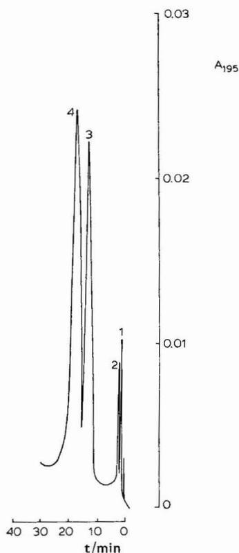
Fig. 3. Chromatogram of four basic amino acids. Operating conditions: eluent, 0.11 M phosphate buffer; pH 2.0;  $I = 0.2 \text{ mol l}^{-1}$ ; flow-rate;  $1 \text{ ml min}^{-1}$ ; detector, UV. Peaks: 1 = Orn; 2 = Lys; 3 = His; 4 = Arg.
