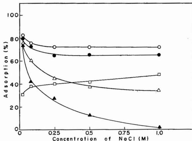
Fig. 3. Effect of salt concentration on the adsorption ratio for proteins. Adsorption was carried out by the method in Fig. 2 except that the pH and salt concentration of the protein solution was varied. Proteins: ●, ovalbumin; ○, serum albumin; □, gelatin; △, pepsin; ▲, lysozyme.
