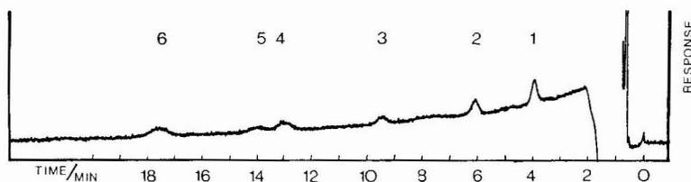
Fig. 2. Chromatogram of a mixture of amines in ethanol with 500 ppm ammonia added. Injection 3  $\mu$ l. Solutes (each 0.1 ppm): 1 = hexylamine; 2 = heptylamine; 3 = octylamine; 4 = benzylamine; 5 = tributylamine; 6 = N,N-dimethylaniline. Attenuation:  $2 \cdot 10^{-12}$  A.f.s. Other conditions as in Fig. 1.
