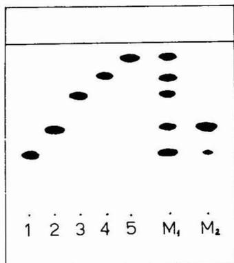
Fig. 1. Thin-layer chromatogram of xanthates of  $C_1$ - $C_5$  aliphatic alcohols on Polygram CEL 400. Solvent: *n*-butanol-water-ammonia solution (5:4:1). Xanthate derivatives from (1) methanol; (2) ethanol; (3) propanol; (4) butanol; (5) amyl alcohol; ( $M_1$ ) mixture of equal amounts of  $C_1$ - $C_5$ -alkanols; ( $M_2$ ) first fraction from distillation of methanol-ethanol-water (1:40:59).
