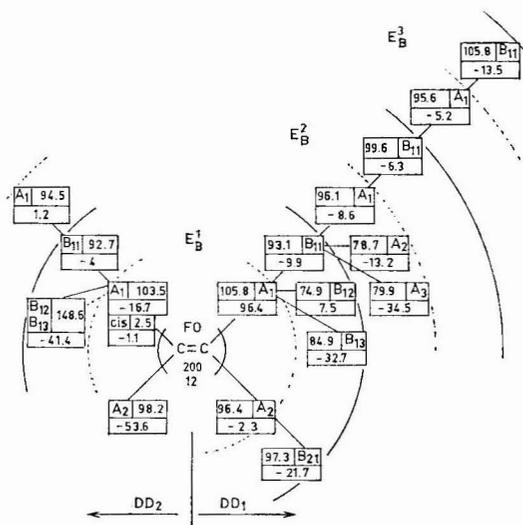
Fig. 8. Extent of specific interactions of alkenes with the nickel form of the ion exchanger. Upper values in each box are retentions on unsulfonated copolymer, lower values are the specific and supplementary contributions due to the nickel form of the ion exchanger.
