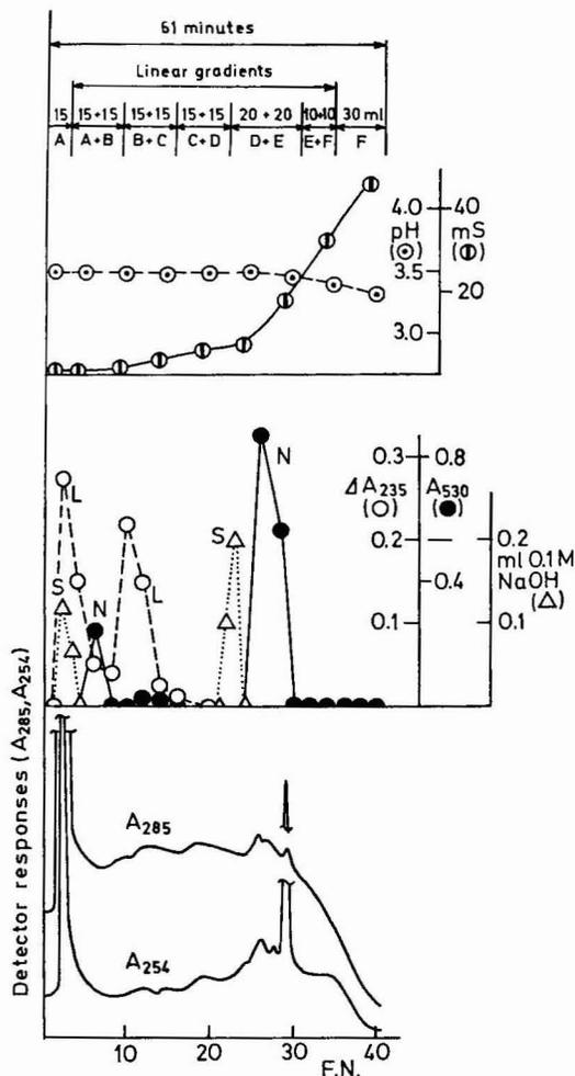
Fig. 4. Chromatography of 25 mg Pectinex Ultra on sulphonated cation exchanger Spheron S-1000. Fractions 4.7 ml per 90 sec; pressure 0.7 MPa. The buffers were prepared from sodium hydroxide of the indicated concentration, adjusted to pH 3.5 with formic acid: A, 0.05 M; B, 0.1 M; C, 0.2 M; D, 0.3 M; E, 0.5 M, 1 M in sodium chloride; F, 2 M sodium chloride. Enzymatic activities as in Fig. 1. F.N. = fraction number.
