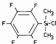
An extremely sensitive derivatizing agent for the analysis of sterols, alcohols, phenols, amines and carboxylic acids by EC-GC:
