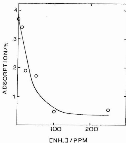
Fig. 8. Adsorption of methylamine on glass surfaces from an ethanolic solution containing various concentrations of ammonia. Concentration of methylamine 0.1 ppm. Temperature: 22°C.
