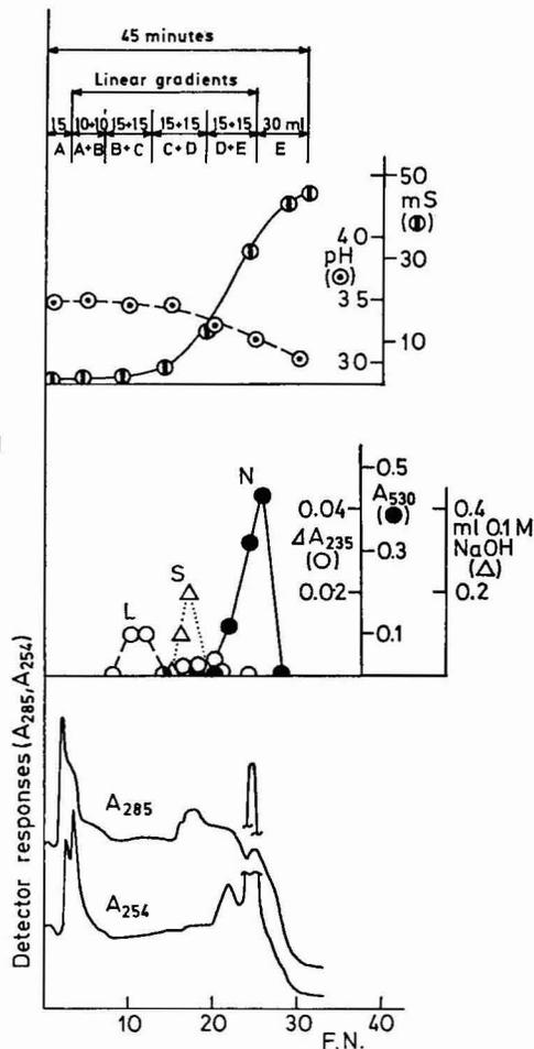
Fig. 10. Chromatography of 25 mg of Rohament P on carboxylated cation exchanger Spheron C-1000. Fractions 4.8 ml per 90 sec; pressure 0.4 MPa. The buffers were identical to those in Fig. 2. Enzymatic activities as in Fig. 1. F.N. = fraction number.
