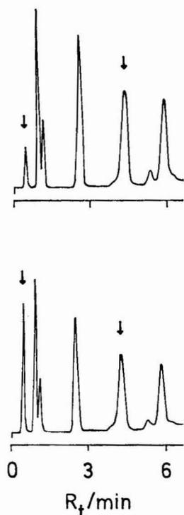
Fig. 6. Pyrograms of OTCS-silica. Top, uncapped material; bottom, capped material. The arrows mark the  $C_1$  and  $C_4$  peaks used for the calculation of the  $C_1/C_4$  peak-height ratios in Table IV. GC system A.
