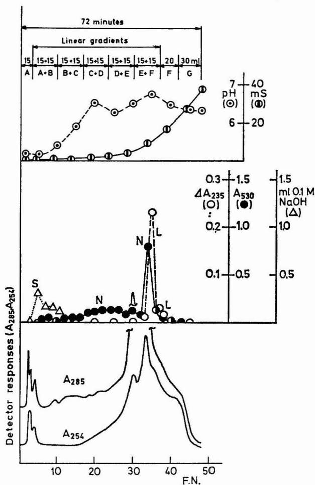
Fig. 6. Chromatography of 25 mg of Pectinex Ultra on Spheron DEAE-1000, on elution with buffers of pH 5. The buffers were prepared as in Fig. 5, but were adjusted to pH 5. Enzymatic activities as in Fig. 1. F.N. = fraction number.
