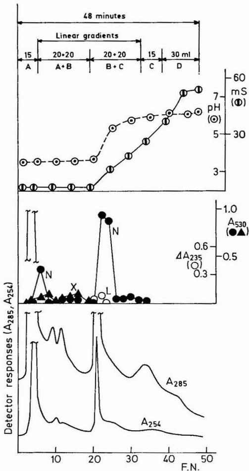
Fig. 12. Chromatography of 25 mg of Rohament P on Spheron Phosphate 1000. Fractions 2.9 ml per 1 min; pressure 0.4 MPa. Buffers A–D as in Fig. 3. Enzymatic activities as in Figs. 1 and 3. F.N. = fraction number.
