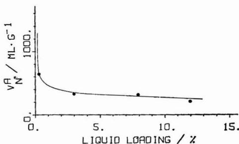
Fig. 2. Adsorption contribution to retention volume of diisopropyl ether *versus* liquid loading of *n*-octadecane for the support B2 (HCl-gas treated).
