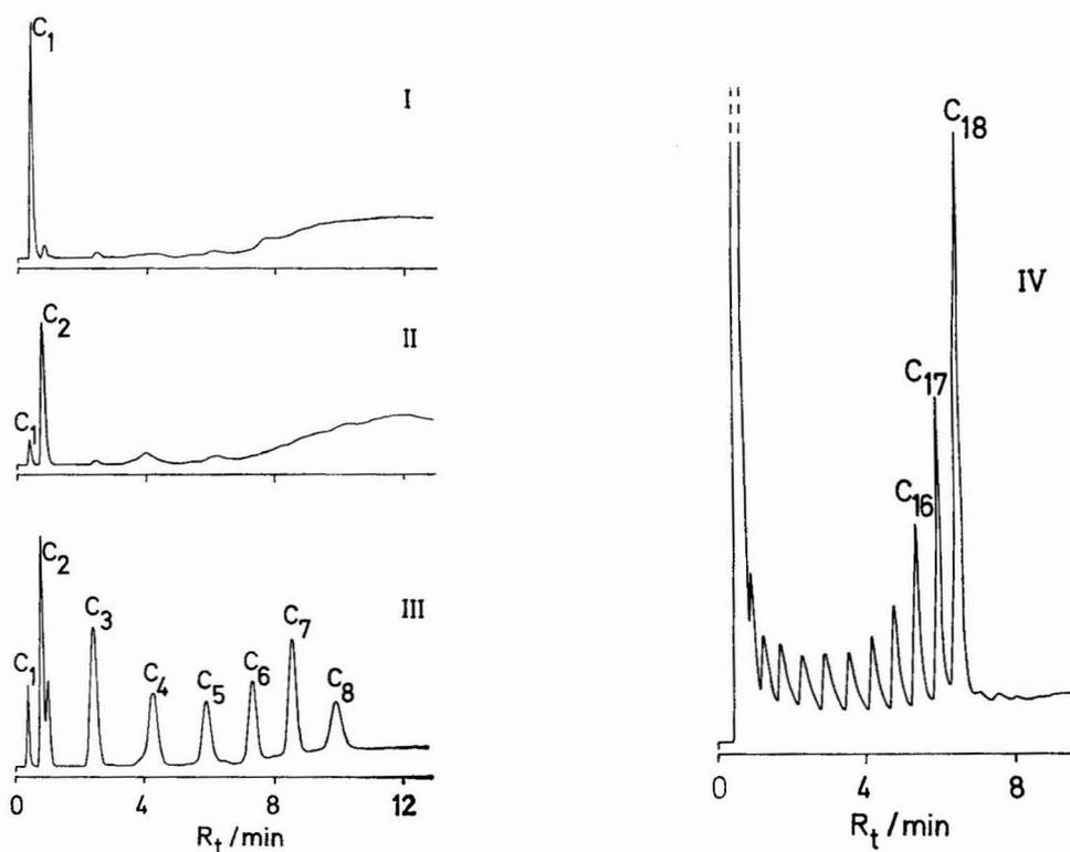
Fig. 3. Pyrograms of CBSPs with different chain length of the hydrocarbon moiety (R). I, R = methyl-, GC system A; II, R = vinyl-, GC system A; III, R = octyl-, GC system A; IV, R = octadecyl-, GC system B. I, II and IV, home-made CBSP; III, LiChrosorb RP-8.
