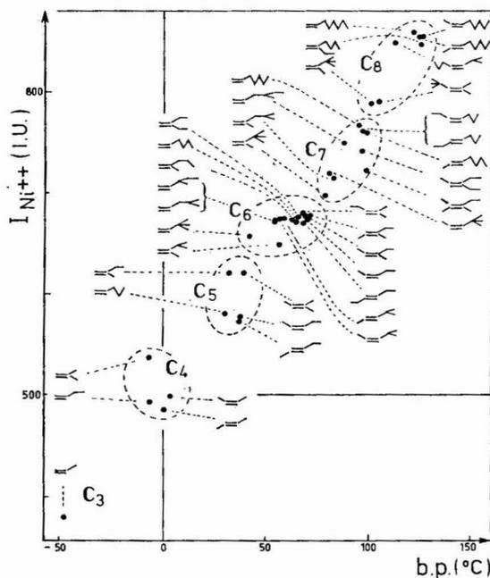
Fig. 7. Retention index of alkenes on the nickel form of the ion exchanger as a function of boiling point of the alkene. The dispersion of the data for each subpopulation suggests, in this instance, a relatively complex law for the structural effects on the adsorption phenomena.
