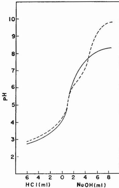
Fig. 1. Titration curve of immobilized tannin. One gram of wet immobilized tannin (-----) or 50 mg of native tannin (—) in 25 ml of water was titrated with 0.01 *N* NaOH or 0.01 *N* HCl using a potentiograph E 336 Metrohm.
