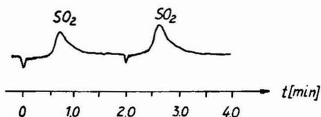
Fig. 4. Determination of SO<sub>2</sub>. Column: 25 cm × 4 mm I.D., glass, deactigel. Carrier gas: air. Temperatures: 130°C; oven, 900°C. Concentration of amine: 20 ppm. Sample size: 1 ml air with 5 ppm SO<sub>2</sub>.
