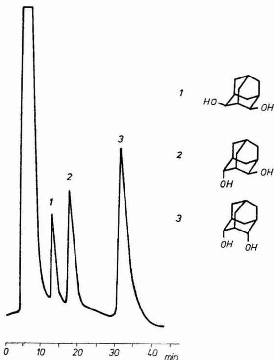
Fig. 1. Separation of the three adamantane-2,4-diol stereoisomers. Column, MicroPak CH-10; mobile phase, methanol-water (20:80); flow-rate, 10 ml/h; temperature, 30°C.
