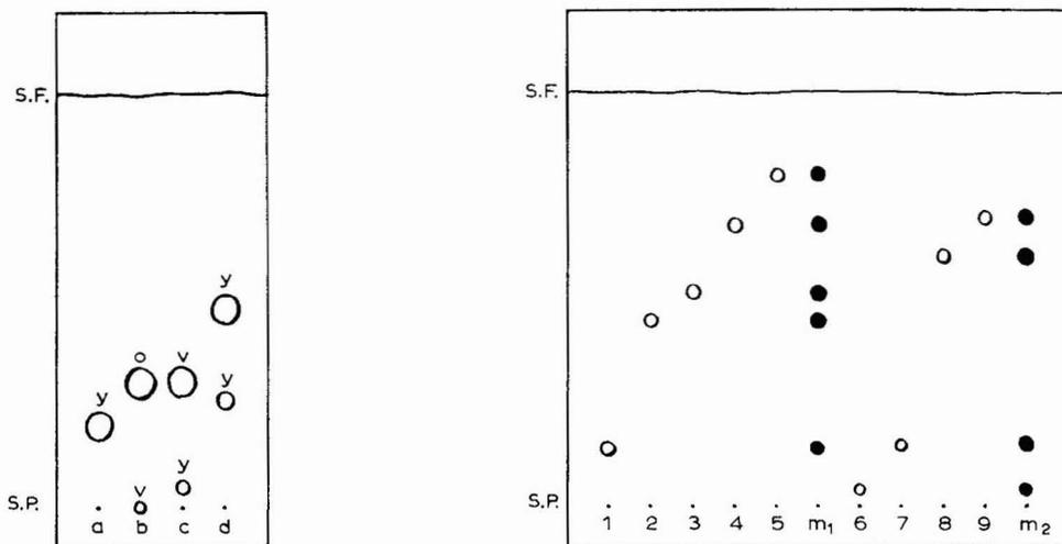
Fig. 1. Thin-layer chromatogram of standard solutions of amines, 10 days after their preparation, on  $\text{AWP}:\text{CaSO}_4 \cdot \frac{1}{2}\text{H}_2\text{O}$  in the ratio 4:2. Eluent: 1 *M* nitric acid. Amines (1  $\mu\text{g}$ ): a = *m*-nitroaniline; b = *p*-nitroaniline; c = *o*-nitroaniline; d = *p*-aminobenzoic acid. Colours after spraying with *p*-DAB: y = yellow; o = orange; v = violet. S.P. = Starting point; S.F. = solvent front.
