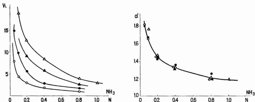
Fig. 2. Retention volumes of L-leucine as a function of ammonia concentration in the eluent. Degree of saturation of the L-hydroxyproline resin by  $\text{Cu}^{2+}$ :  $\Delta$ , 100%;  $\blacktriangle$ , 88%;  $\bullet$ , 70%;  $\circ$ , 59%. Sample: 1 mg of L,D-Leu. Chromatographic conditions as in Fig. 1.
