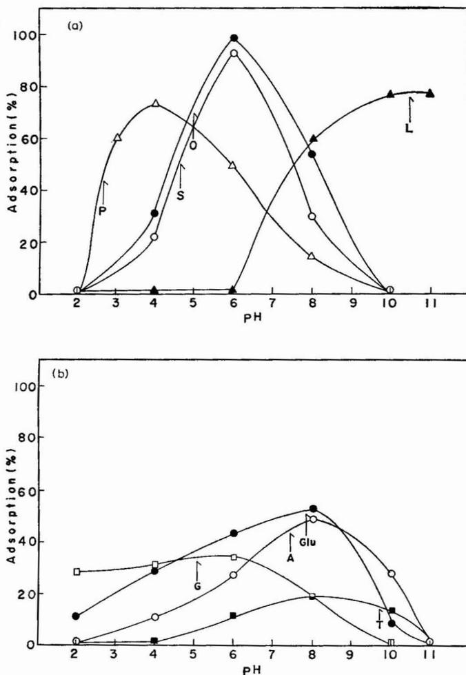
Fig. 2. Effect of pH on adsorption ratio for proteins. Adsorption was carried out by shaking 200 mg (wet weight) of immobilized tannin with 10 ml of 0.1% protein dissolved in the following buffer solutions: pH 2, 0.01 *N* HCl; pH 3-5, 0.01 *M* acetate buffer; pH 5-8, 0.01 *M* phosphate buffer; pH 9-11, 0.01 *M* carbonate buffer. The adsorption ratios were calculated from:
