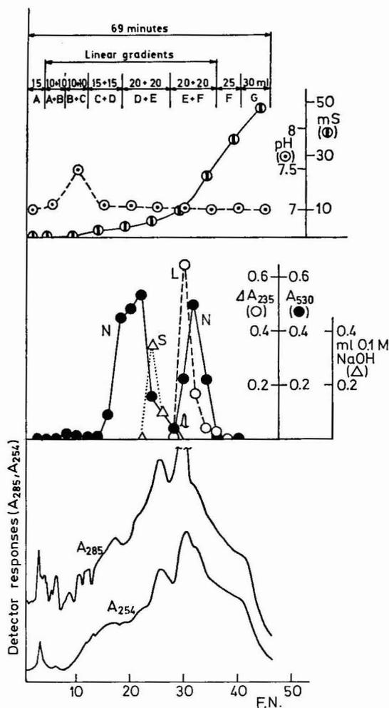
Fig. 8. Chromatography of 25 mg of Pectinex Ultra on strongly basic anion exchanger Spheron TEAE-1000. Fractions 4.6 ml per 90 sec; pressure 0.6 MPa. The buffers of pH 7 were identical to those in Fig. 5, and the labelling of enzymatic activities is also the same. F.N. = fraction number.
