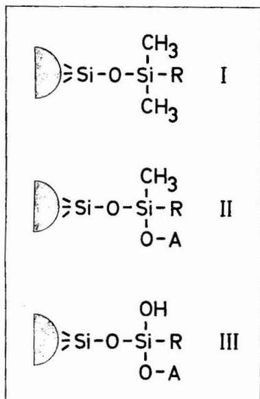
Fig. 2. Schematic formulae of the different structures of CBSPs obtained when mono- (I), di- (II) and tri- (III) functional silanizing agents are reacted with the silica surface. R = Hydrocarbon chain; A = H or Si→.
