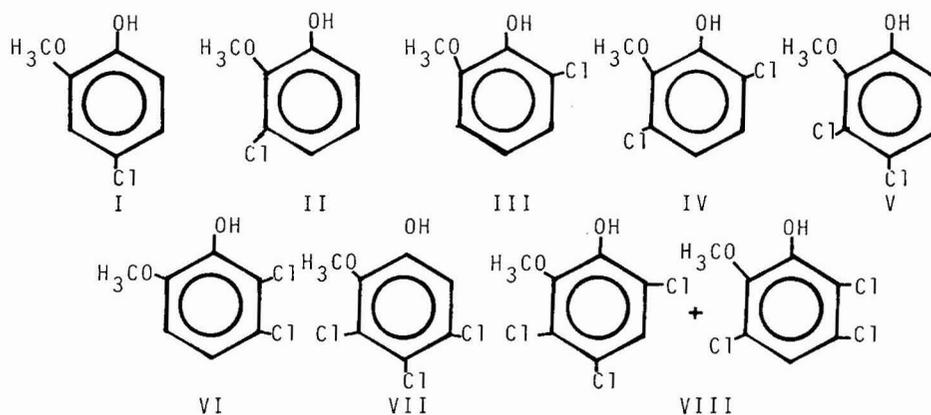
Fig. 1. Structures of 4-chloroguaiacol (I), 3-chloroguaiacol (II), 6-chloroguaiacol (III), 3,6-dichloroguaiacol (IV), 3,4-dichloroguaiacol (V), 5,6-dichloroguaiacol (VI), 3,4,5-trichloroguaiacol (VII) and a mixture (1:1) of 3,4,6-trichloroguaiacol and 3,5,6-trichloroguaiacol (VIII).
