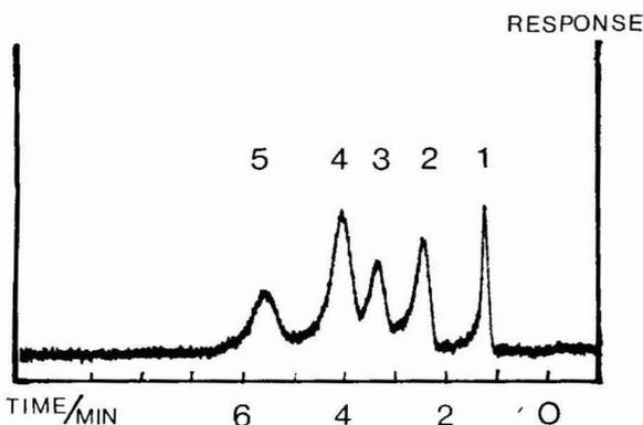
Fig. 6. Chromatogram from injection of  $3 \mu\text{l}$  of a mixture of volatile amines in water. Solute concentration  $0.1 \text{ ppm}$ . Solutes: 1 = ammonia; 2 = methylamine; 3 = dimethylamine; 4 = ethylamine; 5 = isopropylamine. Temperature:  $60^\circ\text{C}$ . Attenuation:  $1 \cdot 10^{-12}$  A.f.s. Other conditions as in Fig. 1.
