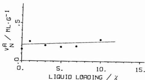
Fig. 3. Adsorption contribution to retention volume of methanol *versus* liquid loading of *n*-octadecane for support B3 (Carbowax-modified).
