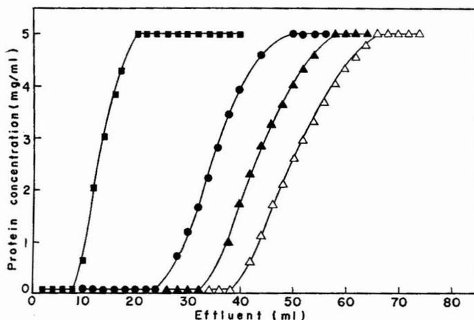
Fig. 4. Adsorption capacity of immobilized tannin for proteins. Buffer solutions for equilibration of the column were 0.05 M acetate buffer, pH 4, for pepsin; 0.05 M acetate buffer, pH 6, for ovalbumin; 0.05 M phosphate buffer, pH 8, for trypsin; and 0.05 M carbonate buffer, pH 10, for lysozyme. Other conditions are given in the text. Proteins: ■, trypsin; ●, ovalbumin; ▲, lysozyme; △, pepsin.
