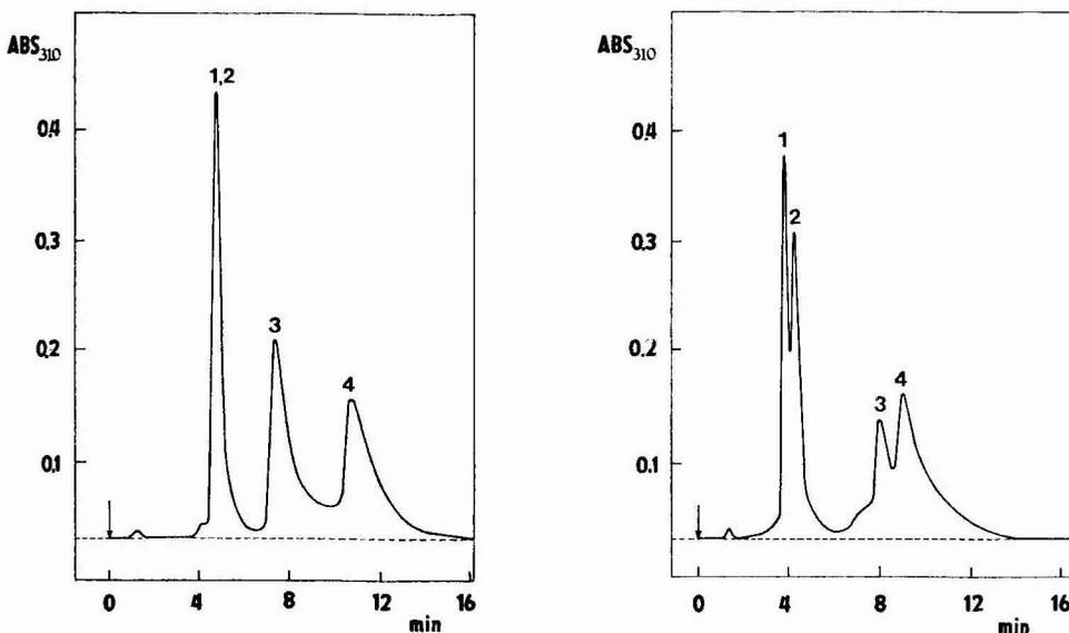
Fig. 3. Chromatogram of mixture of diastereomeric pairs of ergocornine and ergocornam. Column, LiChrosorb  $NH_2$ ; mobile phase, diethyl ether–ethanol (96:4); flow-rate of the mobile phase, 40 ml/h; pressure, 2.5 MPa; detector, Variscan UV at 310 nm. Peaks: 1 and 2 = ergocorninam and ergocorninine; 3 = ergocornine; 4 = ergocornam.
