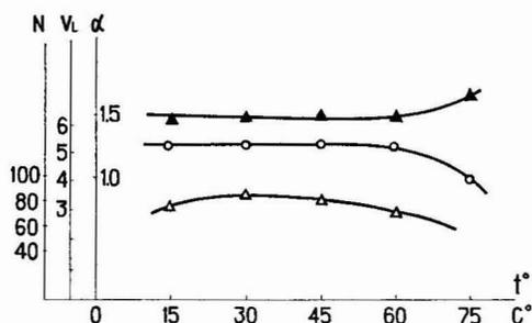
Fig. 4. Chromatography of 1.2 mg L,D-Leu showing temperature dependence of the number of effective plates,  $N$  ( $\Delta$ ) enantioselectivity,  $\alpha$  ( $\blacktriangle$ ) and the retention volume of L-Leu,  $V_L$  ( $\circ$ ). Column:  $140 \times 9$  mm. Eluent:  $0.2 N$   $NH_4OH$ ; flow-rate 35 ml/h.
