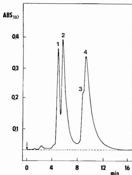
Fig. 2. Chromatogram of a mixture of diastereomeric pairs of ergocristine and ergocristam. Column, LiChrosorb NH<sub>2</sub>; mobile phase, diethyl ether-ethanol (96:4); flow-rate of the mobile phase, 40 ml/h; pressure, 2.5 MPa; detector, Variscan UV at 310 nm. Peaks: 1 = ergocristinam; 2 = ergocristinine; 3 = ergocristine; 4 = ergocristam.
