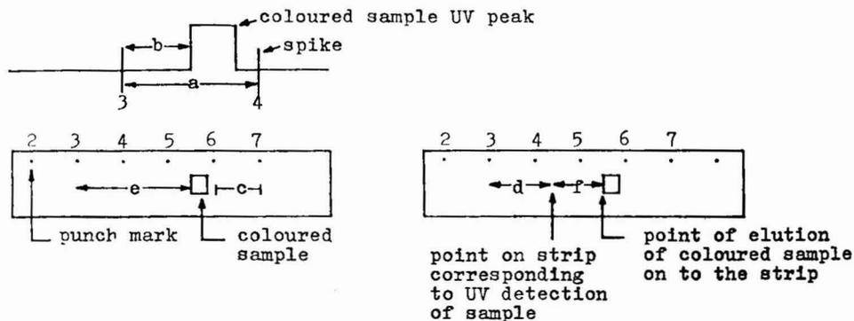
Fig. 2. Scheme for determination of  $f$  value.
