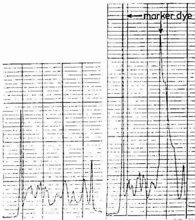
Fig. 3. Comparison of the same diagram region of two runs carried out with and without dye. Although the dye produces mixed zones with sample components, the other components are not effected.
