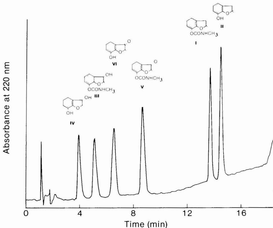
Fig. 3. Chromatogram of carbofuran and its five metabolites. Packing: Zorbax ODS. Column: 25 cm  $\times$  4.6 mm I.D. Mobile phase: as described in Experimental, 1.5 ml/min (System B); recorder sensitivity, 0.116 absorbance units full scale; injection volume, 10  $\mu$ l. Concentration of standards ( $\mu$ g/ml). I, 57.8; II, 61.3; III, 41.8; IV, 36.4; V, 37.3; VI, 28.9.
