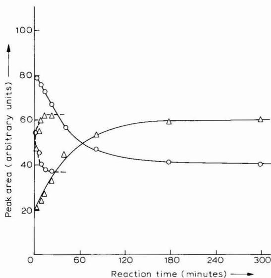
Fig. 1. Time required for equilibrium between  $\alpha$ -glucose (O) and  $\beta$ -glucose ( $\Delta$ ) at 22°C: —, a freshly prepared solution of glucose in water; ---, the same solution but after addition of 0.001 M triethylamine.
