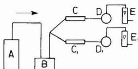
Fig. 1. Schematic diagram of apparatus. A = Reactor; B = refrigerator; C, C<sub>1</sub> = adsorbent beds; D, D<sub>1</sub> = suction pumps; E, E<sub>1</sub> = flow meters.
