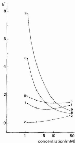
Fig. 9. Influence of concentration of buffer ions on column capacity ratios. Stationary phase: Partisil-10 SCX cation exchanger. Mobile phase: triethylammonium formate-75% acetonitrile (pH 3.0). Solutes: 1 = cAMP; 2 = N<sup>6</sup>-monobutyl-cAMP; 5 = 8-dimethylamino-cAMP; 8 = adenosine; 9 = adenine.
