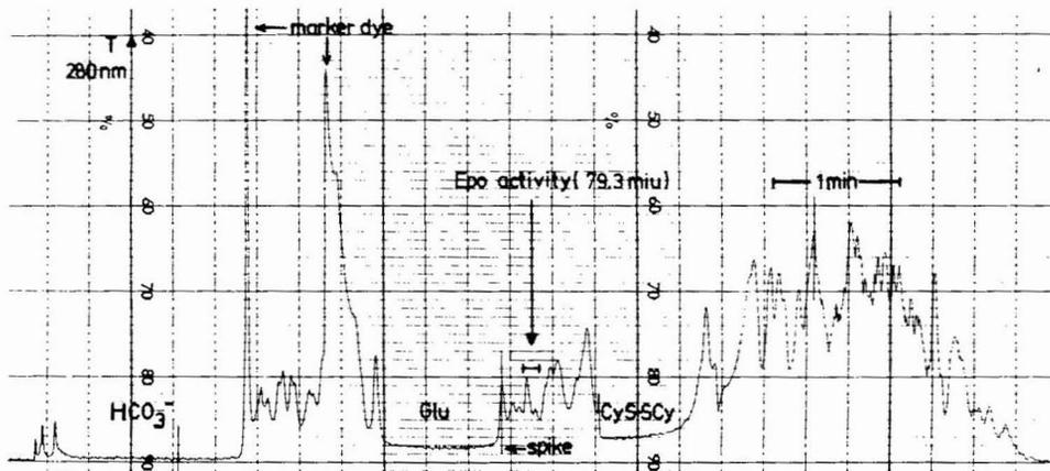
Fig. 4. UV diagram of a fractionation run. Glu and (Cys)<sub>2</sub> were used as discrete spacers. Erythropoietin activity could be detected only in the peak region marked.
