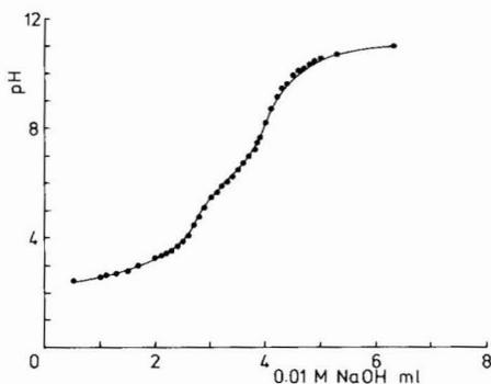
Fig. 9. Titration curve obtained with APBA-Sepharose (CNBr-activated). Samples of gel were washed with distilled water and the pH adjusted to a value of 2.5 with dilute HCl. The suspension was then titrated with 0.01 *M* NaOH with constant stirring under nitrogen. The titration was carried out at room temperature. Ligand concentration 8 mg APBA per ml gel (wet weight).
