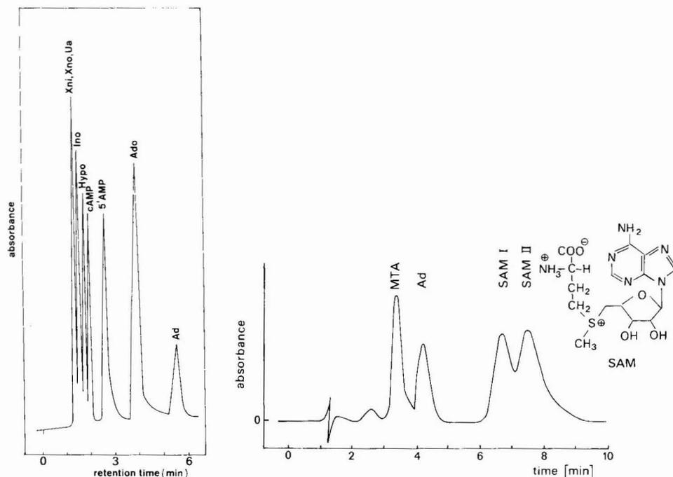
Fig. 13. Separation of cyclic AMP and its enzymatic degradation products by mixed chromatography. Stationary phase: Partisil-10 SCX cation exchanger. Mobile phase: 3 mM triethylammonium formate–67% acetonitrile (pH 3.0); flow-rate, 3 ml/min. Solutes: Xni = xanthine; Xno = xanthosine; Ua = uric acid; Ino = inosine; Hypo = hypoxanthine; cAMP = adenosine-3',5'-monophosphate; Ado = adenosine; Ad = adenine.
