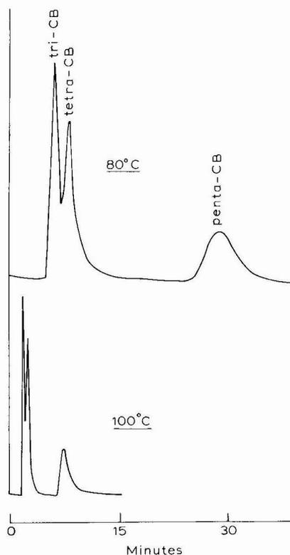
Fig. 2. Chromatograms of 2',3,4-trichlorobiphenyl (tri-CB), 2,2',5,5'-tetrachlorobiphenyl (tetra-CB) and 2,2',4,4,5,5'-pentachlorobiphenyl (penta-CB) on a 1-m Apolane-87 capillary column at 80 and 100°C.
