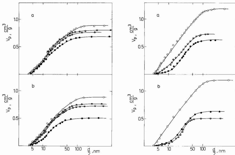
Fig. 1. Integral distribution curves of pore sizes of copolymers 1-6. (a) Effect of the time of thermal treatment: ○, copolymer 1 (original); ●, copolymer 2 (250°C, 1 h); ●, copolymer 3 (250°C, 2 h); ●, copolymer 4 (250°C, 4 h). (b) Effect of temperature: ○, copolymer 1 (original); ●, copolymer 3 (250°C, 2 h); ●, copolymer 5 (260°C, 2 h); ●, copolymer 6 (280°C, 1 h).
