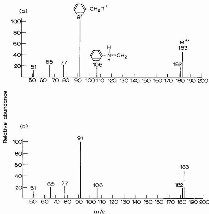
Fig. 2. Mass spectra of (a) synthetic N-benzylaniline and (b) metabolically produced N-benzylaniline.
