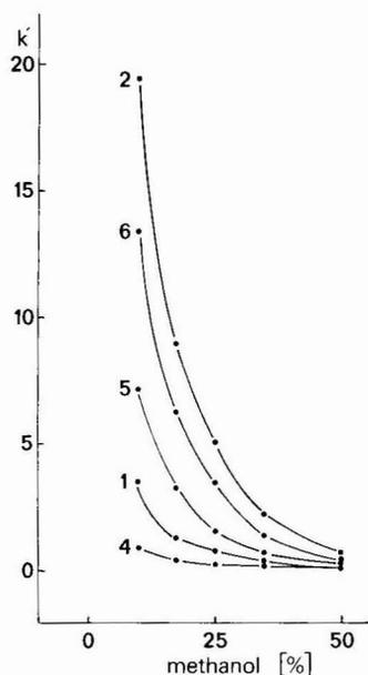
Fig. 2. Influence of methanol concentration on column capacity ratios. Mobile phase: 10 mM tributylammonium formate (pH 3.0). Solutes (see Table I): 1 = cAMP; 2 = N<sup>6</sup>-monobutyl-tyr-yl-cAMP; 4 = 8-amino-cAMP; 5 = 8-dimethylamino-cAMP; 6 = 8-benzylamino-cAMP.
