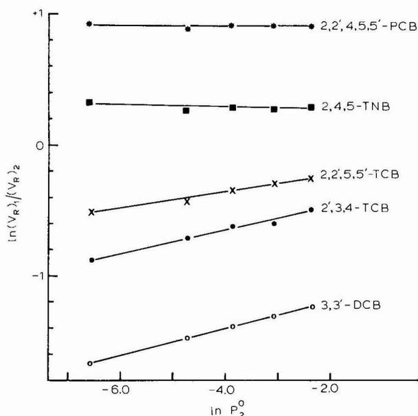
Fig. 1. Plots of  $\ln(V_R)_1/(V_R)_2$  vs.  $\ln p_2^0$  (vapor pressure of 2,4,5-TIB at different temperatures) for PCB isomers and 2,4,5-trichlorophenoxyacetic acid, *n*-butyl ester (2,4,5-TNB).
