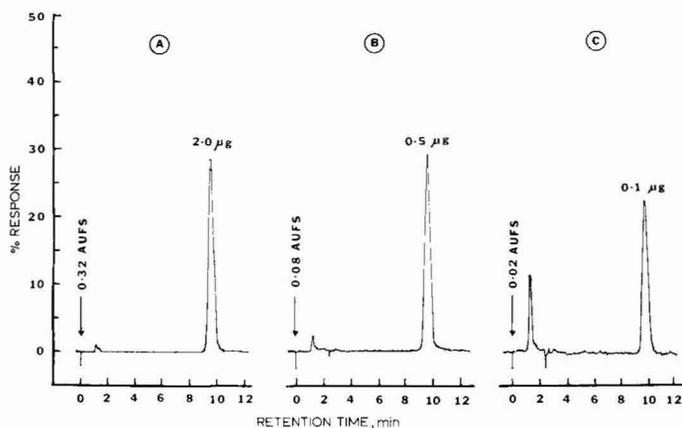
Fig. 2. HPLC chromatogram tracings of cyclohexanone oxime standards; (a) 2.0  $\mu\text{g}$ , (b) 0.5  $\mu\text{g}$ , (c) 0.1  $\mu\text{g}$ . Elution solvent, acetonitrile-water (1:3); flow-rate 1 ml/min.
