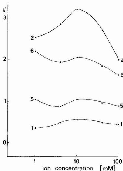
Fig. 4. Influence of concentration of buffer ions on column capacity ratios. Mobile phase: 30% methanol-tributylammonium formate (pH 3.0). Solutes: (see Table I): 1 = cAMP; 2 = N<sup>6</sup>-monobutyryl-cAMP; 5 = 8-dimethylamino-cAMP; 6 = 8-benzylamino-cAMP.
