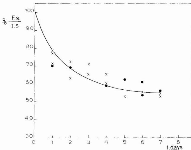
Fig. 2. Loss by polymerization of styrene vapour (percentage of final styrene, F.s., with respect to initial styrene, I.s.) with time. Adsorbent carbon size: x, 15-30 mesh; ●, 30-100 mesh.
