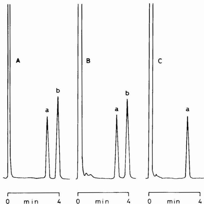
Fig. 2. Gas chromatograms of 1-*m*-chlorophenylpiperazine heptafluorobutyrate (b) and internal standard (a) from spiked brain sample (A), from brain of rats treated with trazodone (B) and from drug-free brain (C).
