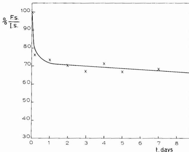
Fig. 3. Loss by polymerization of styrene in solution with time.
