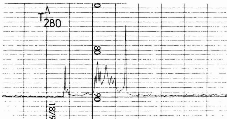
Fig. 1. Buffer run using 1.5  $\mu$ l of 1% Ampholine, pH 3.5–9.5. No effect on detection is observed.
