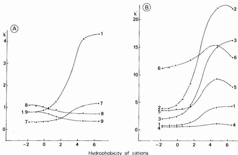
Fig. 5. Influence of the hydrophobicity of the cations on column capacity ratios. Abscissa: hydrophobicity of the cations, calculated with hydrophobic fragmental constants<sup>34</sup>. Cations from left to right on each curve: ethanolammonium, ammonium, monoethylammonium, diethylammonium, triethylammonium, tributylammonium and tetrabutylammonium. Mobile phase: 10% methanol–10 mM cations (pH 3.0), adjusted with formic acid. Solutes: see Table I and Fig. 1.
