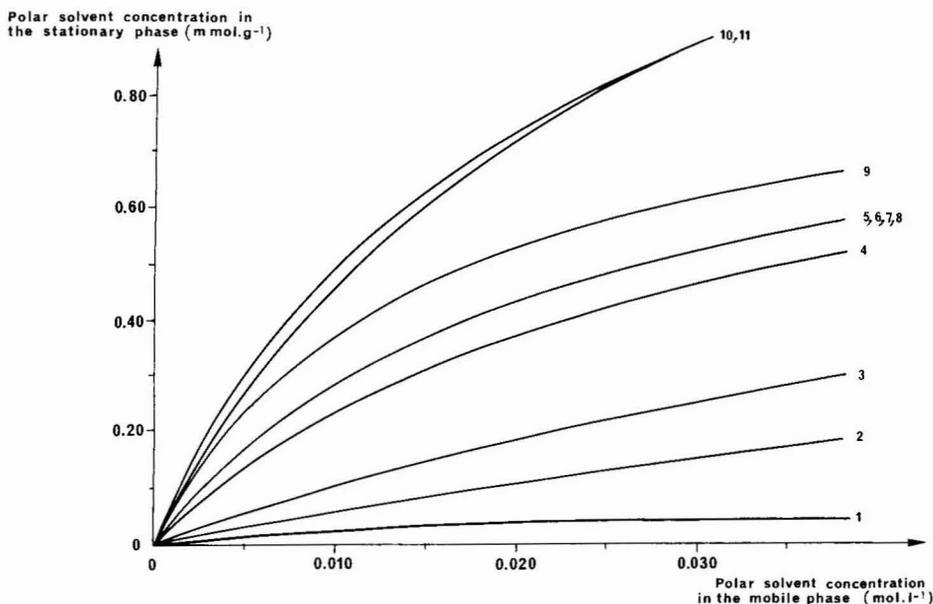
Fig. 1. Adsorption isotherms of polar solvents on LiChrosorb-NH<sub>2</sub> containing 0.9 mmol · g<sup>-1</sup> of amino chains. Solvents: 1, chloroform; 2, nitromethane; 3, acetone; 4, N,N-dimethylformamide; 5, 1-decanol; 6, 1-octanol; 7, 1-pentanol; 8, 1-propanol; 9, ethanol; 10, methanol; 11, benzylmethanol.
