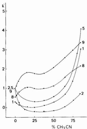
Fig. 5. Influence of polarity of the mobile phase on column capacity ratios. Stationary phase: Partisil-10 SCX cation exchanger. Mobile phase: 5 *M* triethylammonium formate (pH 3.0). Solutes: 1 = cAMP; 2 = N<sup>6</sup>-monobutyryl-cAMP; 5 = 8-dimethylamino-cAMP; 8 = adenosine; 9 = adenine.
