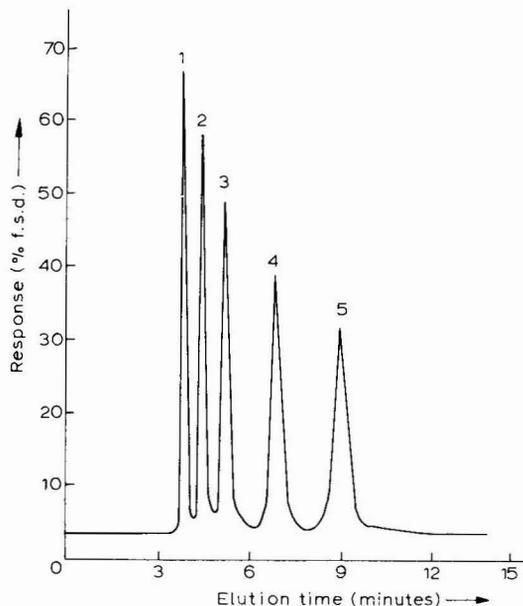
Fig. 3. Chromatogram of glucose (1), mannose (2), fructose (3), mannitol (4) and glucitol (5) under standard conditions.
