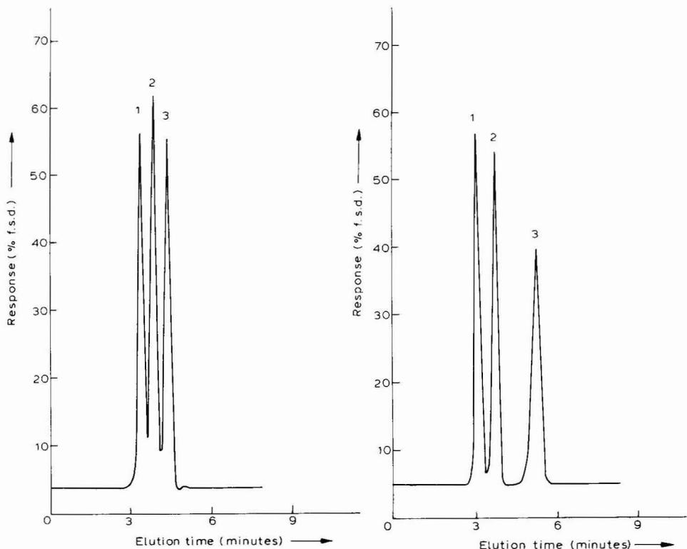
Fig. 4. Chromatogram of lactose (1), glucose (2) and galactose (3) under standard conditions, but with a column temperature of 55°C.
