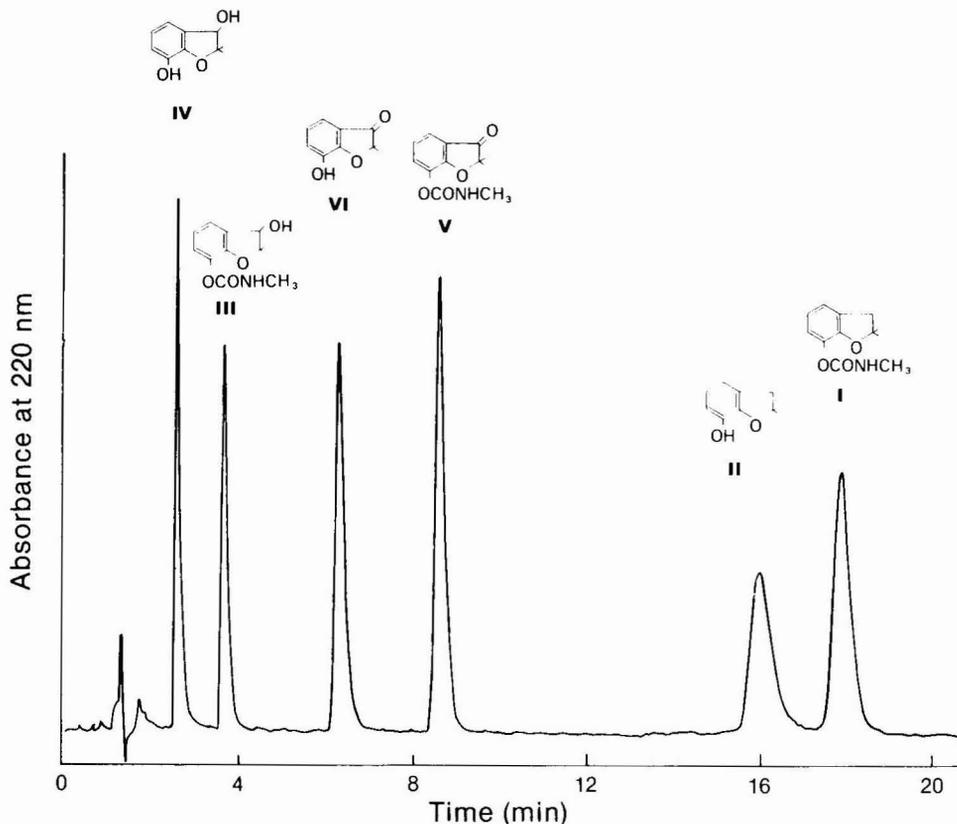
Fig. 2. Chromatogram of carbofuran and its five metabolites. Packing: Zorbax ODS. Column: 25 cm  $\times$  4.6 mm I.D. Mobile phase: acetonitrile–water (25:75), 2 ml/min (System A); recorder sensitivity, 0.058 absorbance units full scale; injection volume, 10  $\mu$ l. Concentration of standards ( $\mu$ g/ml): I, 44.4; II, 48.0; III, 20.0; IV, 40.0; V, 31.6; VI, 12.6.
