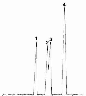
Fig. 1. Chromatogram of hippuric acid (1), *m*-methylhippuric acid (2), *p*-methylhippuric acid (3) and benzoylproline (internal standard) (4).
