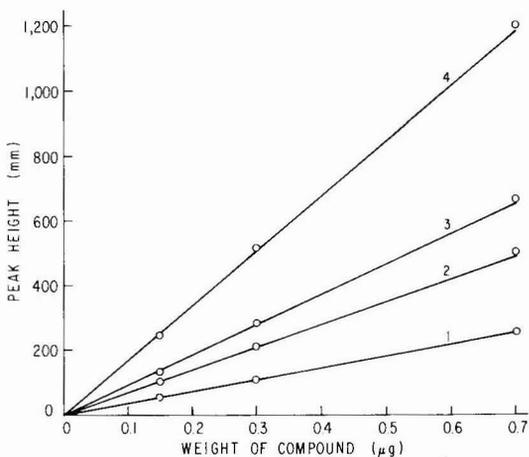
Fig. 4. Standard curves, lubimin (1), rishitin (2), phytuberin (3), and katahdinone (4). HPLC, methanol-water (70:30), 1.0 ml/min, reversed-phase  $\mu\text{Bondapak C}_{18}$  column (30 cm  $\times$  3.9 mm I.D.).
