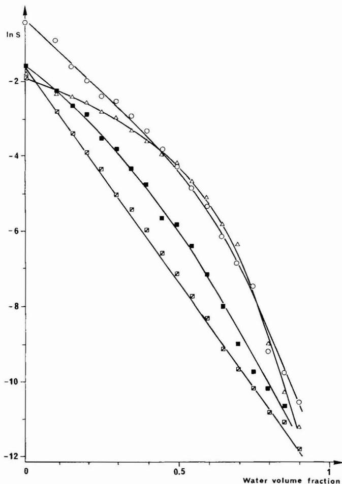
Fig. 8. Variation of logarithm of solubility ( $\text{mole} \cdot \text{l}^{-1}$ ) of phenanthrene in water-organic solvent mixtures with the volume fraction of water. □, Methanol; ○, acetonitrile; ■, ethanol; △, 1-propanol.
