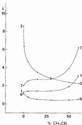
Fig. 4. Influence of polarity of the mobile phase on column capacity ratios. Stationary phase: Partisil-10 SAX anion exchanger. Mobile phase: 20 mM triethylammonium formate (pH 3.0). Solutes: 1 = cAMP; 2 = N<sup>6</sup>-monobutryryl-cAMP; 6 = 8-benzylamino-cAMP; 7 = 5'-AMP.
