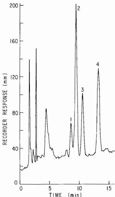
Fig. 2. High-performance liquid chromatogram of authentic sesquiterpenes: lubimin (1), rishitin (2), phytuberin (3), and katahdinone (4) ( $0.2 \mu\text{g}$  of each compound). Methanol-water (70:30), 1.0 ml/min, wavelength 200 nm, 0.02 a.u.f.s., reversed-phase  $\mu\text{Bondapak C}_{18}$  column (30 cm  $\times$  3.9 mm I.D.).
