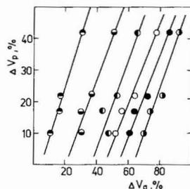
Fig. 3. Effect of decrease in the specific pore volume of samples obtained by the thermal treatment of copolymer 1 on the reduction of the retention volumes of sorbates; ○, pentane; ●, heptane; ●, nonane; ●, benzene; ●, propanol; ●, nitromethane.
