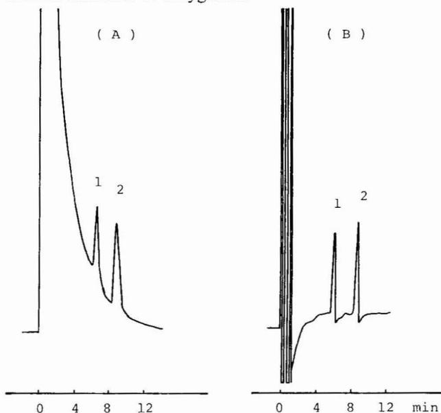
Fig. 1. Gas chromatogram of benzaldehyde produced from hydrolysis of amygdalin by  $\beta$ -glucosidase on a 2.0-m 3% GE-XE column at 160°C. 1 = Benzaldehyde O-pentafluorobenzoyloxime; 2 =  $\alpha,\alpha$ -dichlorodiphenylmethane. (A) Analysis on a gas chromatograph equipped with a hydrogen FID, using 2.0  $\mu$ g of amygdalin. (B) Analysis on a gas chromatograph equipped with a  $^{63}\text{Ni}$  ECD, using 200 ng of amygdalin.
