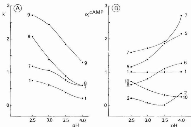
Fig. 10. Influence of pH on column capacity ratios (A) and selectivity to cAMP (B). Stationary phase: Partisil-10 SCX cation exchanger. Mobile phase: 5 mM triethylammonium formate-65% acetonitrile. Solutes: 1 = cAMP; 2 = N<sup>b</sup>-monobutryl-cAMP; 5 = 8-dimethylamino-cAMP; 6 = 8-benzylamino-cAMP; 7 = 5'-AMP; 8 = adenosine; 9 = adenine; 10 = 8-bromo-cAMP.
