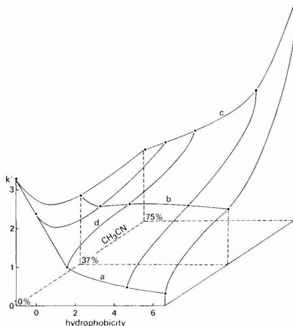
Fig. 11. Influence of hydrophobicity of the buffer ions and polarity of the mobile phase on column capacity ratios of adenosine. Stationary phase: Partisil-10 SCX cation exchanger. Mobile phase: 5 mM cations (pH 3.0). Cations used: ammonium, ethylammonium, triethylammonium, tributylammonium and tetrabutyl ammonium. Their hydrophobicities were calculated with the hydrophobic fragmental constant<sup>44</sup>. For (a) (b), (c) and (d), see text.
