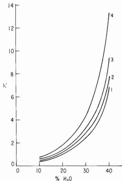
Fig. 3.  $k'$  values obtained for lubimin (1), rishitin (2), phytuberin (3), and katahdinone (4). Methanol-water system, reversed-phase  $\mu\text{Bondapak C}_{18}$  column (30 cm  $\times$  3.9 mm I.D.)  $k' = (t_R - t_{R_0})/t_{R_0}$ , where  $t_{R_0}$  is the retention time of the solvent front, and  $t_{R_1}$  is the retention time of the compound.
