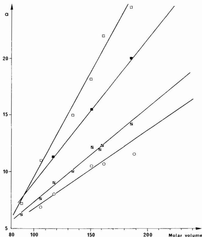
Fig. 7. Variation of the coefficient  $a$  obtained from  $\ln k' = ax^n + b$  with the molar volume of aromatic compounds for different organic modifiers. Experimental conditions as in Fig. 6. □, Methanol; ○, acetonitrile; ■, ethanol; ▲, tetrahydrofuran.
