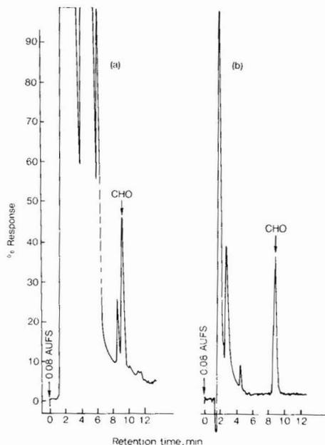
Fig. 4. Chromatogram tracings of urine (a) and plasma (b) spiked to 50  $\mu$ g/ml with cyclohexanone oxime (CHO). Spiked plasma samples were diluted 1:1 with acetonitrile to precipitate the proteins. The peak (retention time 8.5 min) immediately preceding CHO was not observed in all urine samples.
