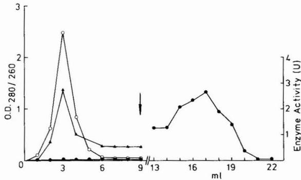
Fig. 6. Chromatography of yeast G-6-PDH by  $\text{NADP}^+$ -presaturated Matrex gel-PBA. Yeast enzyme concentrate (7.5 mg in 0.5 ml) in buffer (ligand concentration,  $41 \mu\text{moles/ml}$ ) (see Fig. 5) was applied to a column of Matrex gel PBA (1 ml) preequilibrated as described in Fig. 5. The concentrate contained 19.4 U of G-6-PDH. Fractions (1 ml) were collected and assayed for enzyme activity (●), O.D. 260 (▲) and O.D. 280 (○). Elution was effected with 2 mM  $\text{NADP}^+$  (arrow).
