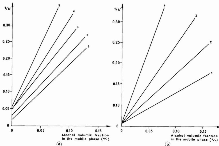
Fig. 4. (a) Variation of  $1/k'$  with volume fraction of methanol in methanol-*n*-hexane mixtures for pyridine derivatives. Flow-rate, 1 ml/min; UV detection at 254 nm. Solutes: 1, 3,4-dimethylpyridine; 2, 4-dimethylpyridine; 3, 3-methylpyridine; 4, 2-methylpyridine; 5, 2,6-dimethylpyridine. (b) Variation of  $1/k'$  with polar modifier concentration in the mobile phase for 2,6-dimethylpyridine. Solutes: 1, 1-octanol; 2, 1-pentanol; 3, 1-propanol; 4, methanol.
