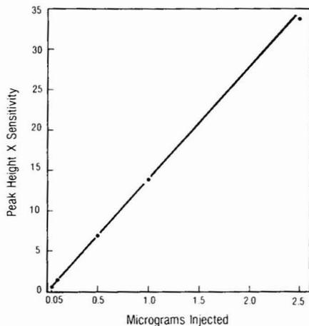
Fig. 3. Linearity, peak height vs. amount of cyclohexanone oxime injected (50 ng–2.5  $\mu$ g).
