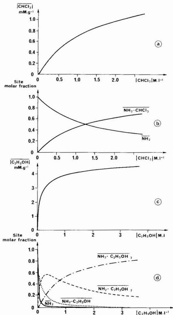
Fig. 2. Adsorption isotherms of chloroform (a) and ethanol (c) on a home-made stationary phase ( $1.1 \text{ mmol}\cdot\text{g}^{-1}$  of amino bonded chains), and computed molar fraction of free and "solvated" groups when varying the polar modifier concentration in the mobile phase: chloroform-*n*-hexane (b) and ethanol-*n*-hexane (d).
