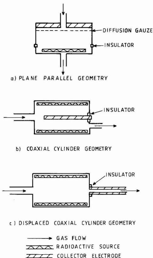
Fig. 1. Schematic diagram of alternative ECD geometries.
