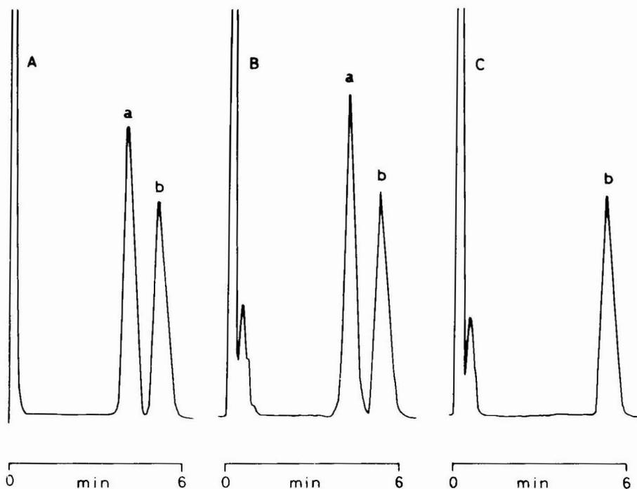
Fig. 1. Gas chromatograms of extracts from spiked brain sample (A), from brain of rats treated with trazodone (B) and from drug-free brain (C). Peaks: (a) trazodone; (b) internal standard.
