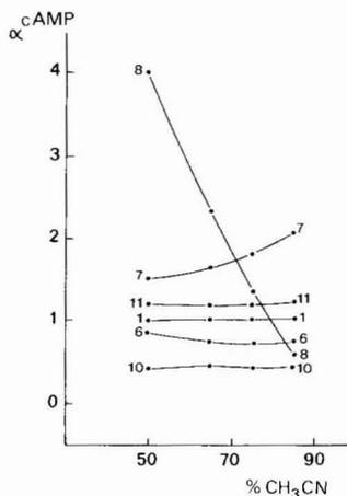
Fig. 8. Influence of polarity of the mobile phase on the selectivity of the solutes to cAMP ( $\alpha^{cAMP}$ ) at high acetonitrile concentrations in the mobile phase. Stationary phase: Partisil-10 SCX cation exchanger. Mobile phase: 5 mM triethylammonium formate (pH 3.0). Solutes: 1 = cAMP; 6 = 8-benzylamino cAMP; 7 = 5'-AMP; 8 = adenosine; 10 = 8-bromo-cAMP; 11 = 8-methoxy-cAMP.
