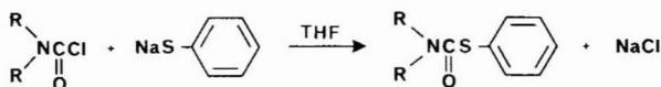
Fig. 1. Structure of distearylcarbamoyl chloride (DACC). On reaction with sodium thiophenolate a stable and UV-absorbing thiocarbamate is formed. R = mainly C 18 H 37 containing about 10% C 16 H 33 and small amounts of C 12 H 25 and C 14 H 29 .
