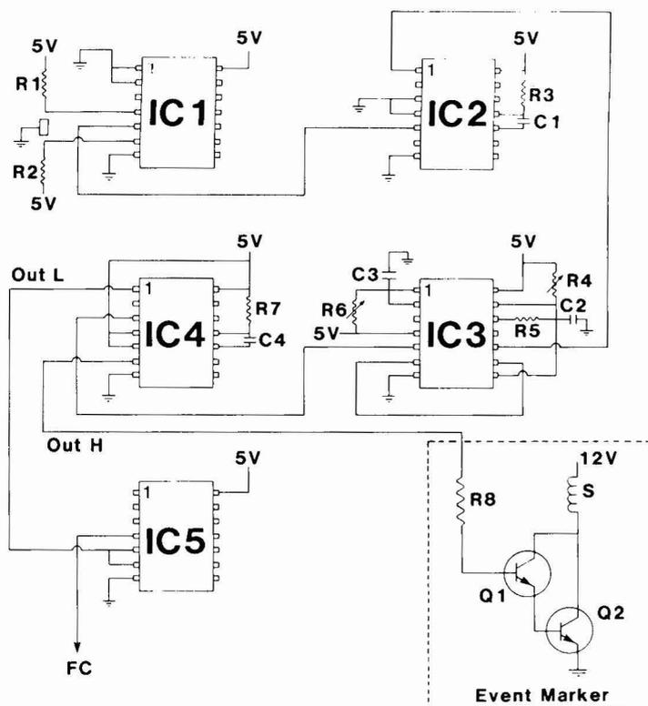
Fig. 1. Circuit diagram. The components were as follows: IC 1 and IC 3, 556 dual timer; IC 2 and IC 4, 74121; IC 5, 7402; Q1 and Q2, 2N2222 transistor; R1, R2 and R7, 10 k $\Omega$ ; R3, 62 k $\Omega$ ; R4 and R6, 1 m $\Omega$  variable; R5, 56  $\Omega$ ; R8, 280  $\Omega$ ; C1 and C4, 10  $\mu$ F; C2, 330  $\mu$ F; C3, 33  $\mu$ F. Out L = output pulse low; Out H = output pulse high; S = event marker solenoid; FC = fraction collector.
