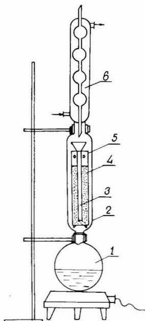
Fig. 1. Modified Soxhlet apparatus for acid washing of the support with the hot extraction acid vapours. 1, Flask (500 cm<sup>3</sup>) with a ground-glass joint; 2, 340 mm × 450 mm I.D. tube with ground-glass joints at both ends; 3, 160 mm × 11 mm I.D. funnel with an elongated tube; 4, Chromosorb P (80–100 mesh); 5, 210 mm × 28 mm I.D. overflow cartridge with three openings for the extraction solution; 6, reflux condenser with ground-glass joint.
