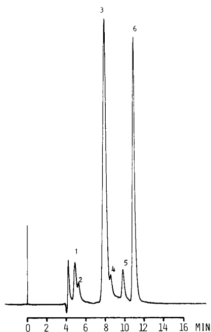
Fig. 8. Separation of oxygen-oxidation products of D-glucose (alkaline solution). Conditions: column, Hamilton HC-X8.00, 10–15 \mu m, 500 \times 9 mm I.D., temperature 80°C; eluent, 0.003 N H 2 SO 4 , flow-rate 1.5 ml/min; UV detection at 210 nm. Peaks: 1 = oxalic; 2 = unknown; 3 = arabinonic; 4 = ribonic; 5 = glycolic; 6 = formic acid.
