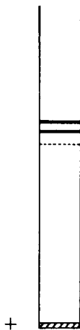
Fig. 2. Distribution of 6-phosphogluconate dehydrogenase after polyacrylamide gel electrophoresis. Purified 6-phosphogluconate dehydrogenase was applied to 7.5% polyacrylamide gels at pH 8.5 and subjected to electrophoresis at 2–3 mA per gel at 4°C for 1–2 h. The figure shows the pattern obtained by subsequent staining for either protein or 6-phosphogluconate dehydrogenase activity.
