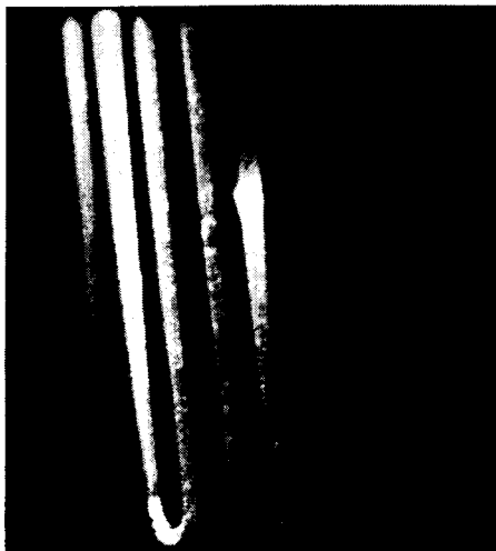
Fig. 7. Inequalities in coating, owing to the thick tullanox layer used.
