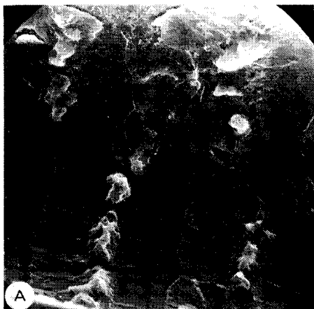
Fig. 7. Scanning electron micrographs ( \times 680 ); A, \text{BaCO}_3 on the wall of a capillary column; B, carbon deposits on the wall of a capillary column.
