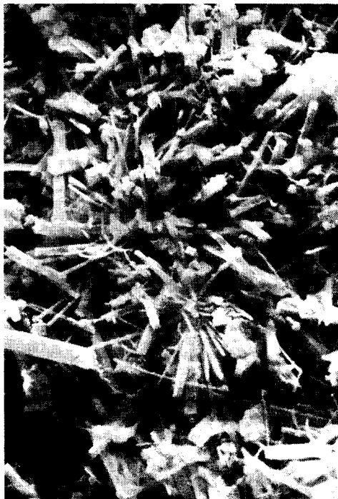
Fig. 17. Macro-crystal forms of aluminosilicate on the surface of support after gas washing (SEM, 5940 \times ).
