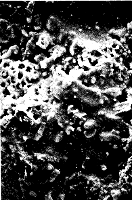
Fig. 13. As Fig. 12: macropores created by production process (SEM, 5940 \times ).
