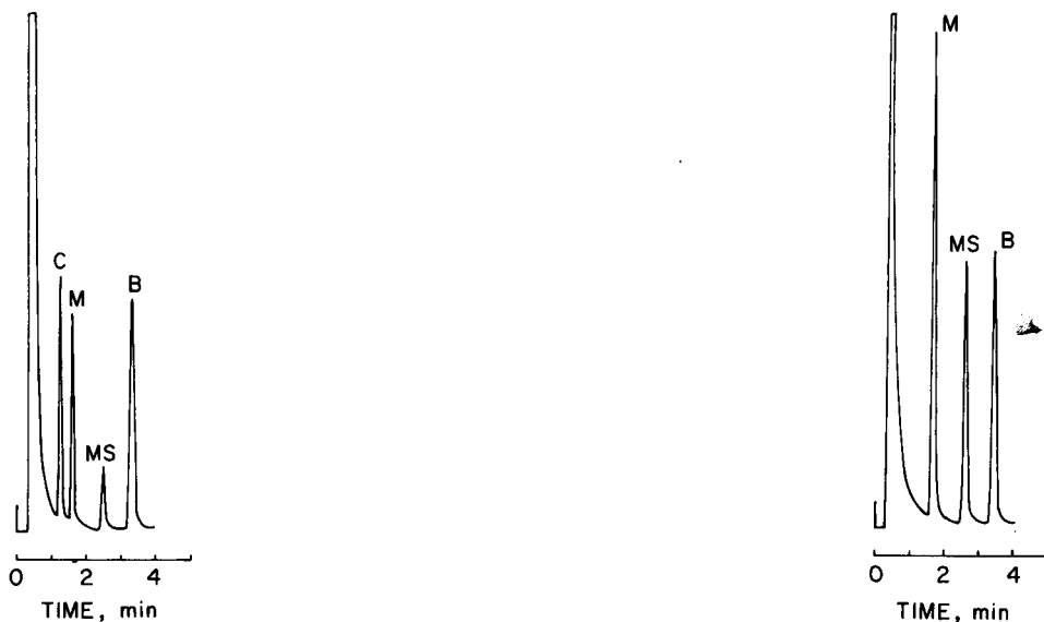
Fig. 3. Gas chromatogram of the extract from a commercial hydrophilic preparation run under conditions described in text. C = camphor; M = menthol; MS = methyl salicylate; and B = benzyl alcohol.
