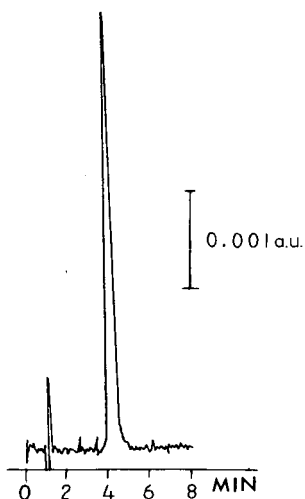
Fig. 1. Chromatogram obtained from plasma containing 100 \mu\text{g/ml} furazolidone and detected at 362 nm. Peak corresponds to 47 ng of furazolidone injected.
