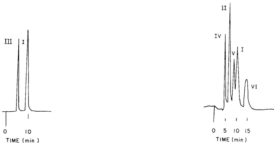
Fig. 4. Reversed-phase ion-pairing chromatogram of mixture of pentazocine hydrochloride (I) and its degradation product pentazocine hydrate (III). Chromatographic conditions given in Fig. 2.
