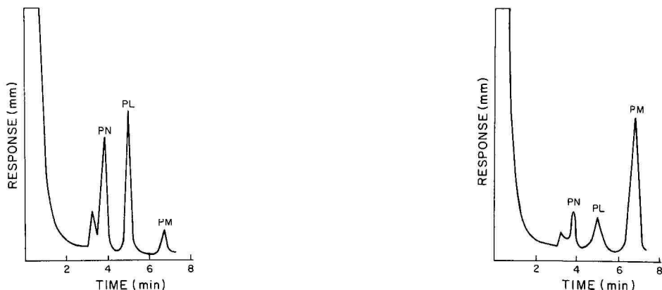
Fig. 1. Separation of B-6 standards by GC-ECD. Conditions: Microtek MT-220; column, 1.54\text{ m} \times 2\text{ mm} I.D., glass, packed with 10% SP-2100 on Supelcoport 80-100 mesh; column, 125^\circ\text{C} , injection port, 205^\circ\text{C} , detector, 350^\circ\text{C} ; carrier gas, nitrogen at 30 ml/min; ^{63}\text{Ni} ECD.
