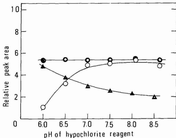
Fig. 2. Effects of pH of hypochlorite reagent on the peak areas: ▲, compound I ( $R = C_{12}H_{25}$ ); ●, II ( $R = C_{12}H_{25}$ ); ○, III ( $R = C_{12}H_{25}$ ). The reaction temperature was fixed at 60°C.
