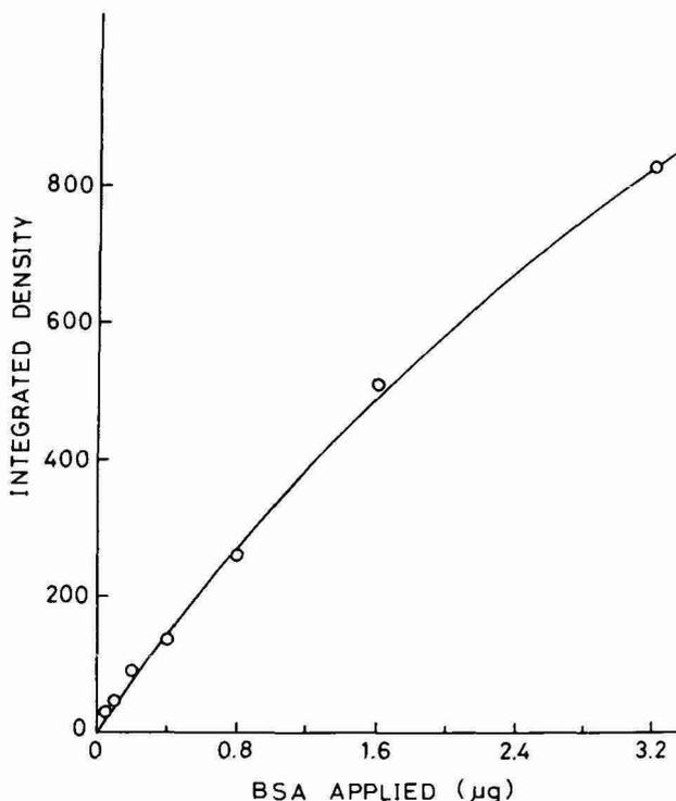
Fig. 5. Integrated density of albumin quantity standard spots. Various amounts of bovine serum albumin, ranging from 0.05 to 3.2  $\mu\text{g}$ , were subjected to micro gradient gel electrophoresis, the gel was stained and the albumin spots were quantitated in  $47 \times 35 \mu\text{m}$  resolution.
