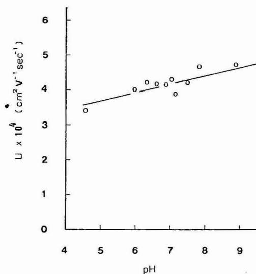
Fig. 3. Effect of pH on electro-osmotic flow. Pyrex glass tubing: 132  $\mu\text{m}$  I.D., length 40 cm from inlet to detector and 10 cm from detector to electrode. Solute: benzene. Solvent: 0.05  $M$  phosphate buffer, pH 7. Constant-voltage mode; 5000 V.
