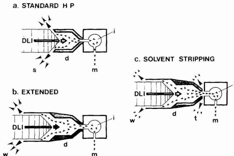
Fig. 3. Schematic diagram showing functioning of the three different DSCs. DLI =  $\mu$ LC probe producing a stream of droplets; d = desolvation chamber; i = ion source; m = ionized stream of solute and solvent molecules focused towards mass filter; s = flow pumped between DSC seat and  $\mu$ DLI probe tip; w = flow pumped through the gap between DSC walls and  $\mu$ DLI probe; t = flow pumped through the gap between DSC tip and ion source body.
