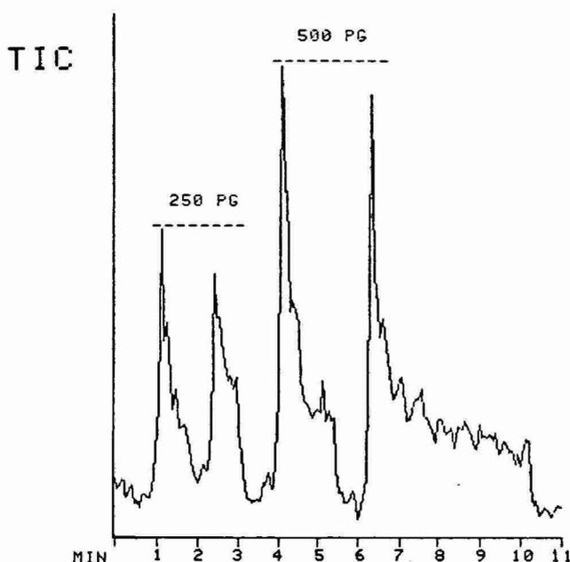
Fig. 7. Negative ion CI  $\mu$ LC-MS total ion current (TIC) profile for repeated injections of 250 and 500 pg of 6-OH- $\beta$ -METH. The  $\mu$ LC-MS eluent/CI reagent gas was methanol-water (65:35) maintained at 40  $\mu$ l/min through a  $C_{18}$  250 mm  $\times$  1 mm I.D. microbore column; solvent-stripping DSC; MS conditions described in Experimental section.
