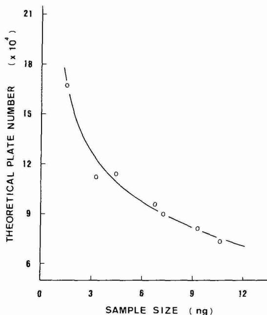
Fig. 4. Relationship between theoretical plate number and sample size. Fused-silica capillary; 72  $\mu\text{m}$  I.D.  $\times$  780 mm, of which 610 mm was used as column. Solvent: 0.02  $M$  phosphate buffer, pH 7, with 0.5% ethylene glycol. Sample: pyridine. Constant-voltage mode: 12.6 kV.
