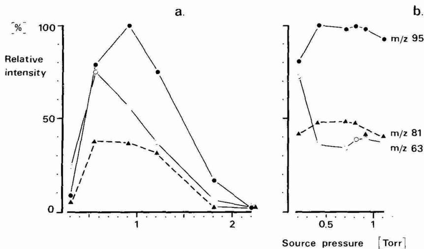
Fig. 5. Plot of the intensity of the three solvent cluster tuning ions versus source pressure, in negative CI at 200°C source and DSC temperature. (a) Extended DSC; (b) solvent-stripping DSC. Intensity normalized according to the most intense value in each DSC; solvent, methanol-water (65:35); flow-rate, 40  $\mu$ l/min.
