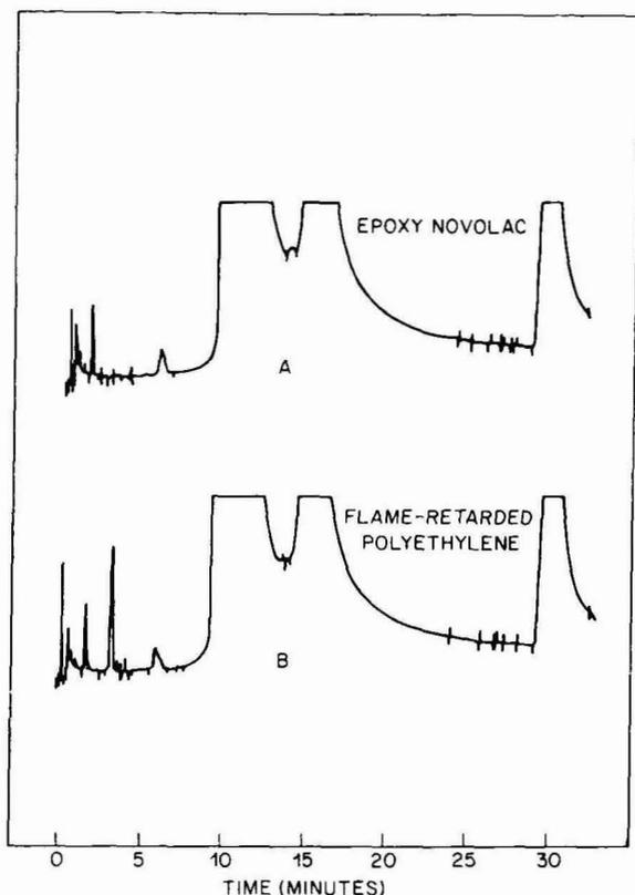
Fig. 3. Chromatograms of derivatized absorbents from burned polymers.
