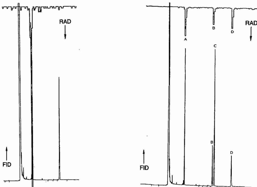
Fig. 8. Chromatogram of  $n\text{-}^{14}\text{C}_{10}$  and  $n\text{-C}_{12}$  hydrocarbons in pentane. Temperature-programmed run:  $110^\circ\text{C}$  isothermal hold 4 min,  $4^\circ\text{C}/\text{min}$  to  $120^\circ\text{C}$  and hold. Durabond 5 J&W,  $30\text{ m} \times 0.32\text{ mm}$  I.D. Absolute recovery of radiolabel under the peak: 80%. RAD efficiency: 68%. Sensitivity: 100 counts full scale. RAD/FID split ratio: 46/54. Mass injected: *ca.* 70 ng per compound.
