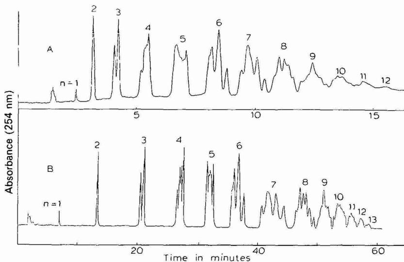
Fig. 1. Chromatograms of 800 MW polystyrene separation on a  $C_{18}$  column with gradient (A), acetonitrile to acetonitrile–methylene chloride (50:50) in 30 min. and (B), acetonitrile–water (80:20, v/v) to acetonitrile in 30 min, held at acetonitrile for 10 min, then changed to acetonitrile–methylene chloride (50:50) in 30 min.
