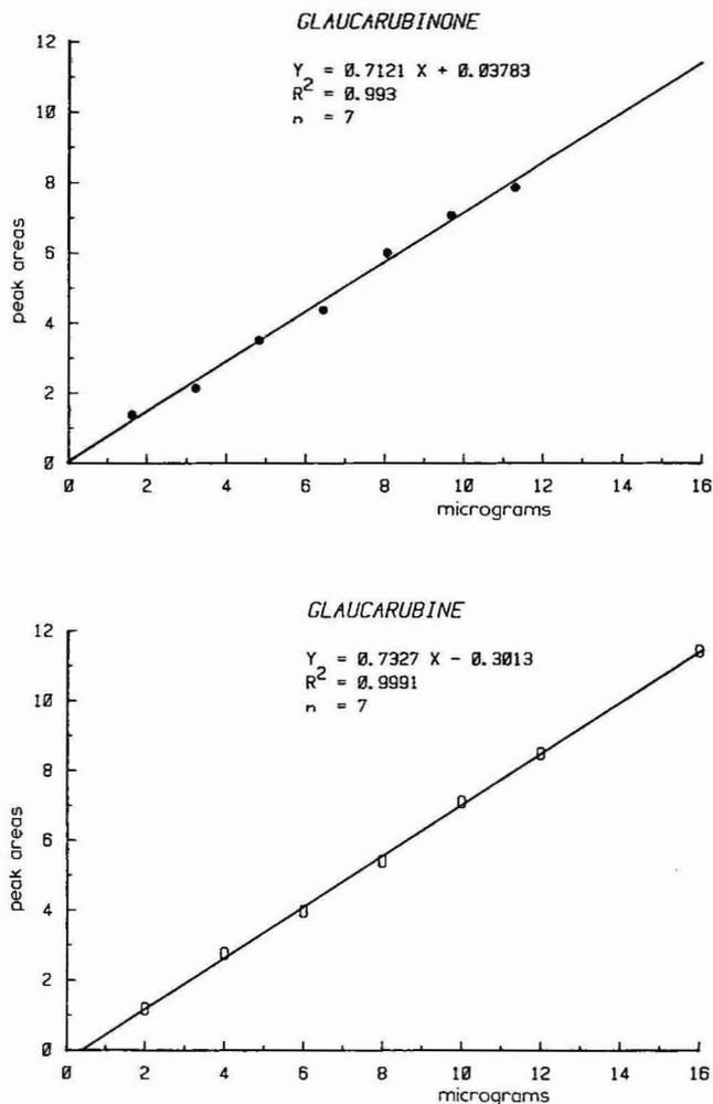
Fig. 2. Calibration curves used for quantitative determination of the concentration of the glaucarubine (O) and glaucarubinone (●) in crude water extracts. The peak areas are linearly correlated with the amount of injected quassinoid.
