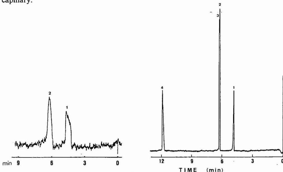
Fig. 6. Separation of cupric (1) and ferric (2) ions. Column: Pyrex glass tubing,  $80 \mu\text{m}$  I.D.  $\times$  36 cm. Solvent:  $0.05 M$  acetic acid. Constant-current mode:  $10 \mu\text{A}$  (ca. 8.6 kV).
