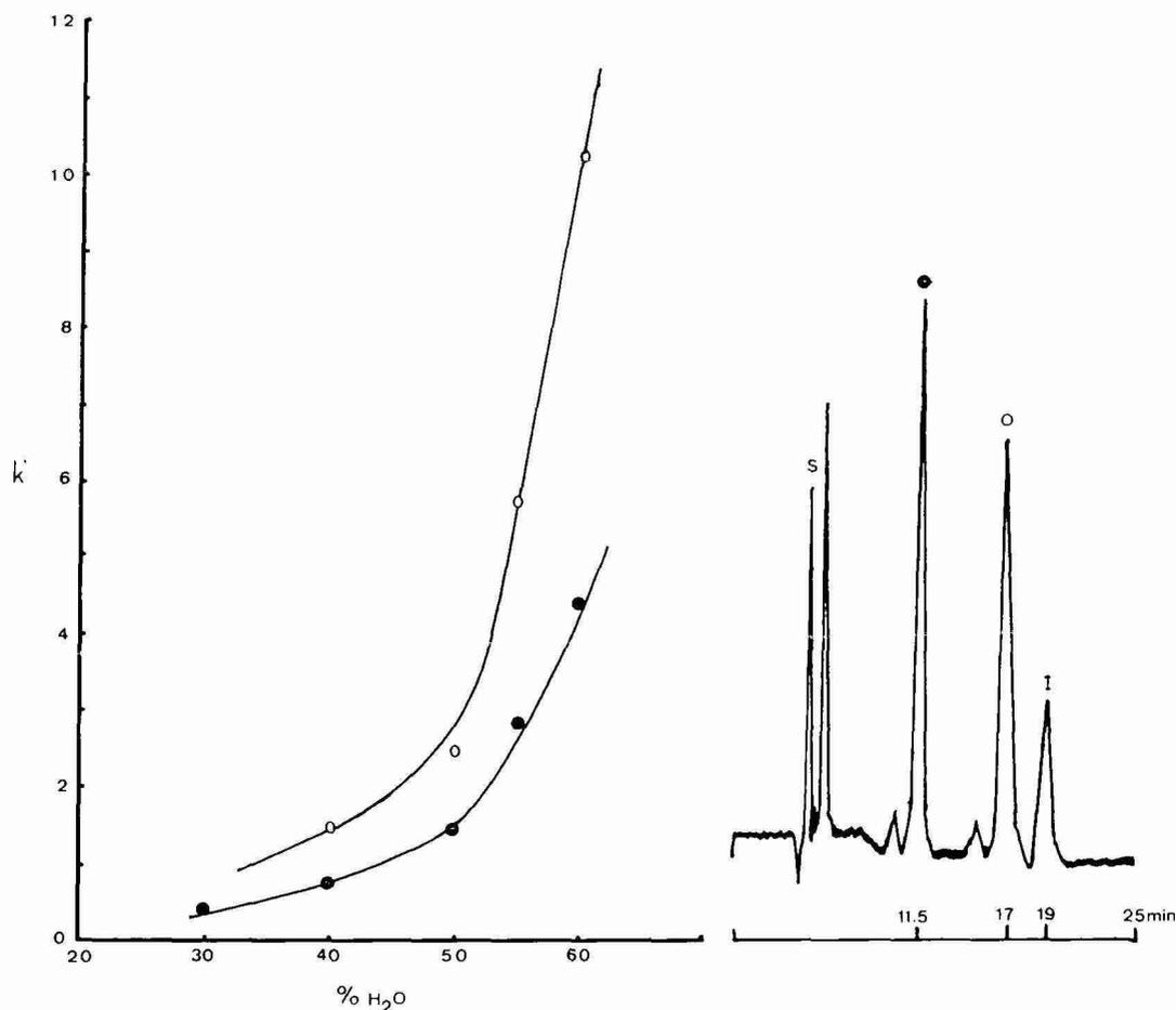
Fig. 3. Capacity factors ( $k'$ ) of glaucarubine (O) and glaucarubinone (●) as a function of the amount of water in the mobile phase.
