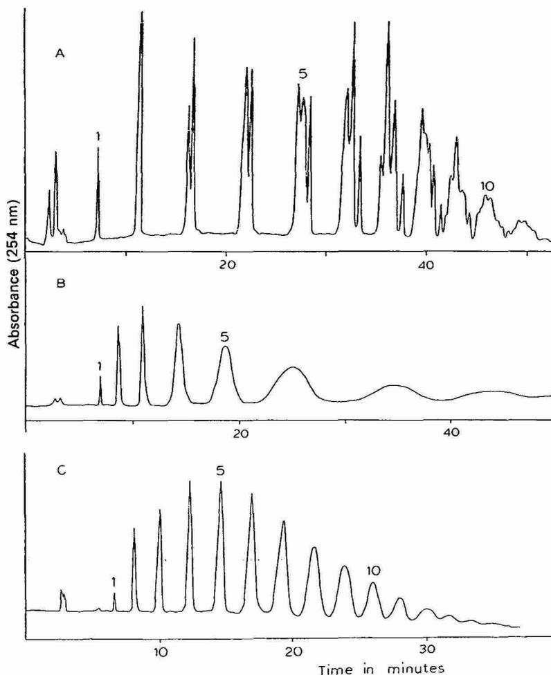
Fig. 8. Chromatogram of the 800 MW polystyrene separation on (A) a  $C_8$  column using gradient (B) in Fig. 1, (B) a fluorinated bonded phase (RPF-10) column holding the mobile-phase composition at acetonitrile-water (60:40), and (C) a phenyl bonded-phase column using a gradient starting at acetonitrile-water (70:30), ramped to acetonitrile-water (90:10) in 30 min and held at this composition until the end of the run.
