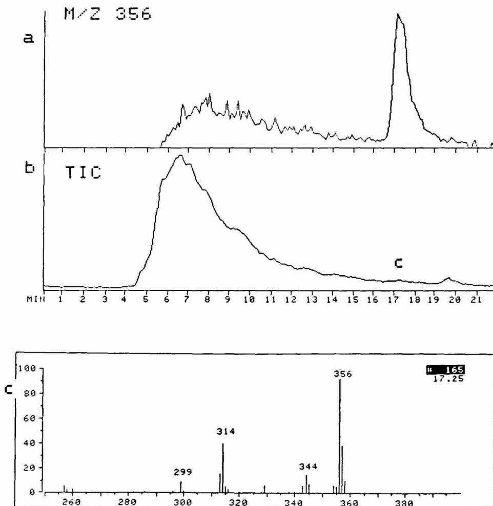
Fig. 8. Negative ion CI  $\mu$ LC-MS analysis of the extract of equine urine collected for 6 h post i.m. administration of 6-Me-PRED. Injection volume, 0.5  $\mu$ l.  $\mu$ LC-MS conditions as in Fig. 7. (a) Reconstructed  $m/z$  356 ion and (b) total ion current profiles; (c) negative CI mass spectrum of 6-Me-PRED, taken at the maximum of the  $m/z$  356 peak in Fig. 8a. Solvent tuning ions ratios:  $m/z$  63:81:95, 47:21:100% relative intensity.
