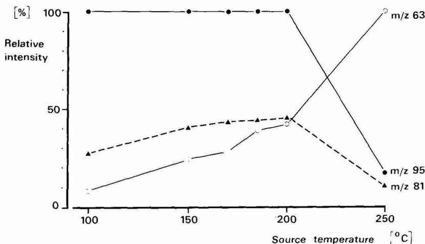
Fig. 6. Plot of the intensity of the three solvent cluster tuning ions versus source temperature, in negative CI at the pressure giving the highest intensity ratio of methanol trimer ion ( $m/z$  95) to methanol dimer ion ( $m/z$  63) with the solvent-stripping DSC. Intensity normalized according to the most intense ion in each measurement; solvent, methanol-water (65:35); flow-rate, 40  $\mu$ l/min.
