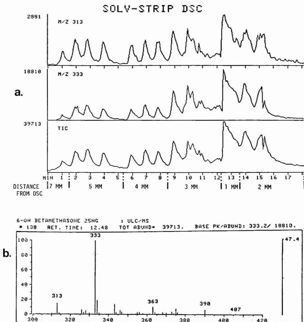
Fig. 4.  $\mu$ LC-MS separation of 6-hydroxybetamethasone (6-OH- $\beta$ -METH) after repeated 25 ng injections; solvent-stripping DSC at 200°C (other standard parameters described in Experimental section). (a) Reconstructed ion chromatograms at different distances of DLI probe in DSC. (b) Mass spectrum recorded at the top of the largest peak ( $t_R = 12.5$  min); solvent tuning ion ratios:  $m/z$  63:81:95, 36:38:100% relative intensity.
