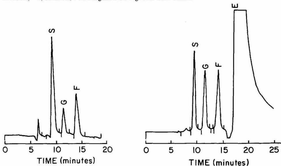
Fig. 3. Typical chromatogram showing quantitative amounts of sucrose, glucose and fructose in low-sugar-type cultivary (37) extracted with warm water (1 g/100 ml). Attenuation,  $\times 2$ ; threshold, 2 for integrator. See Fig. 1 for other details.
