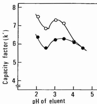
Fig. 4. Effects of eluent pH on  $k'$ . Compounds as in Fig. 2. Eluent: 0.2 M sodium perchlorate containing 60% acetonitrile (pH adjusted by phosphoric acid).
