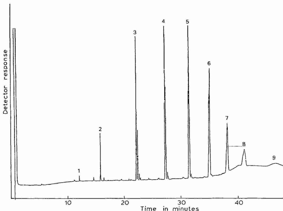
Fig. 10. Capillary GC chromatogram of 666 MW polystyrene separation using a DB-1 column. Column head pressure of  $1.4 \cdot 10^5$  Pa (20 p.s.i.) provided a linear flow-rate of 120 cm/sec. Oven temperature was set at 50°C for 4 min, then ramped at 8°C/min to a final temperature of 350°C.
