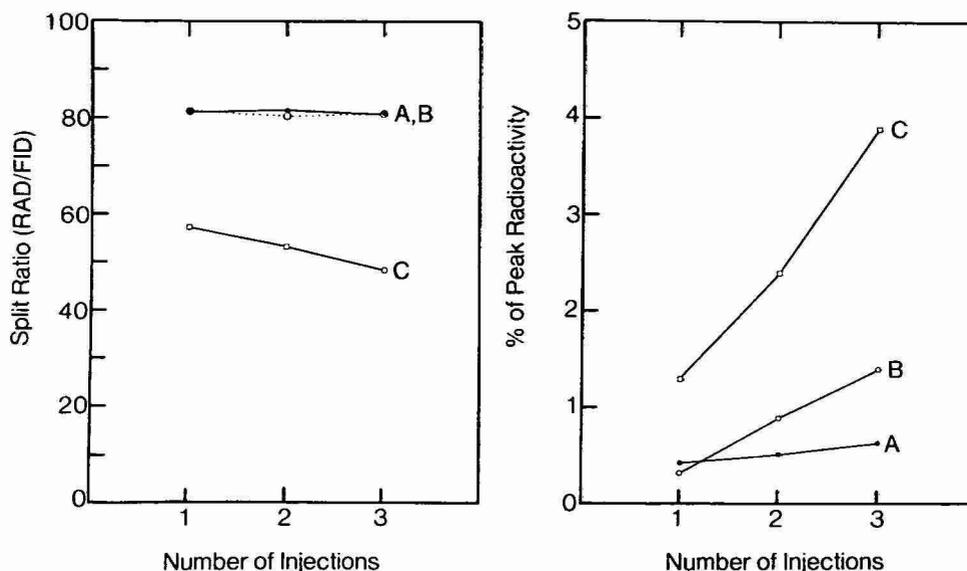
Fig. 5. I, Variation of split ratio after injection of  $^{14}\text{CH}_2\text{Br}_2$ ; II, radioactivity remaining in the combustion tube after injection of  $^{14}\text{CH}_2\text{Br}_2$ . Bed composition: A, CuO: quartz mixture 5:1 (w/w) + a trickle of  $\text{O}_2$ ; B, CuO: quartz mixture 5:1 (w/w) with no added  $\text{O}_2$ ; C, CuO: quartz mixture 3:1 (w/w).
