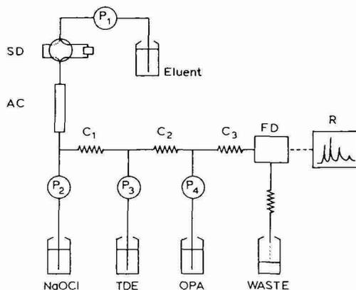
Fig. 1. Flow diagram of the present NaOCl-TDE-OPA post-column derivatization method. SD = Sampling device; FD = fluorescence detector; R = recorder; P<sub>1</sub>-P<sub>4</sub> = pumps; C<sub>1</sub>-C<sub>3</sub> = reaction coils.
