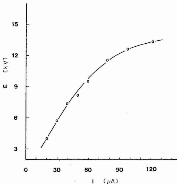
Fig. 1. Relationship between applied voltage,  $E$ , and electric current,  $I$ , under the conditions of zone electrophoresis. Capillary tubing: Pyrex glass capillary (422 mm  $\times$  85  $\mu$ m I.D.) connected with fused-silica capillary (142 mm  $\times$  195  $\mu$ m I.D.). Solvent: 0.02  $M$  phosphate buffer, pH 7, with 0.5% ethylene glycol.
