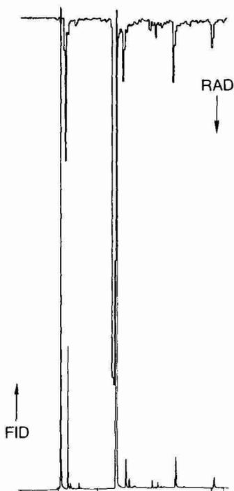
Fig. 10. Chromatogram of underivatized <sup>14</sup>C-diethylenetriamine. Conditions: 140°C isothermal hold 2 min, 8°C/min to 190°C and hold. Carbowax J&W, specially deactivated for amines, 30 m × 0.25 mm I.D. RAD/FID split: 46/54. RAD sensitivity = 1000 counts full scale. Mass (radioactivity) injected = 2 μg (500 nCi).
