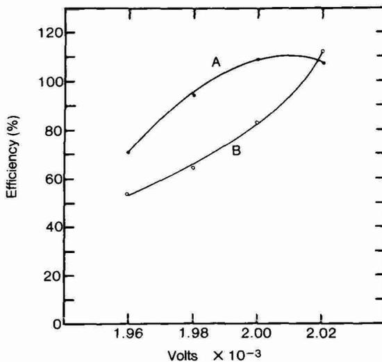
Fig. 7. Counter-tube efficiency as a function of gas composition. A, He 59 ml/min, CO<sub>2</sub> 6 ml/min; B, He 59 ml/min, CO<sub>2</sub> 6 ml/min, O<sub>2</sub> 1 ml/min.
