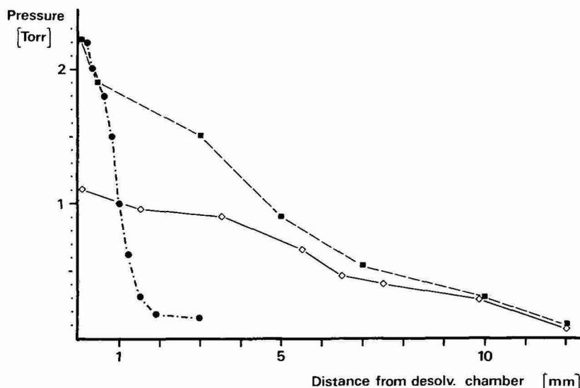
Fig. 2. Plots of ion source pressure *versus* distance between DLI probe tip and seat of desolvation chamber (DSC) for three different DSCs: ●---● = standard Hewlett-Packard DSC; ■---■ = extended DSC; ◇—◇ = solvent-stripping DSC. Solvent methanol-water (65:35); source and DSC temperature, 200°C.
