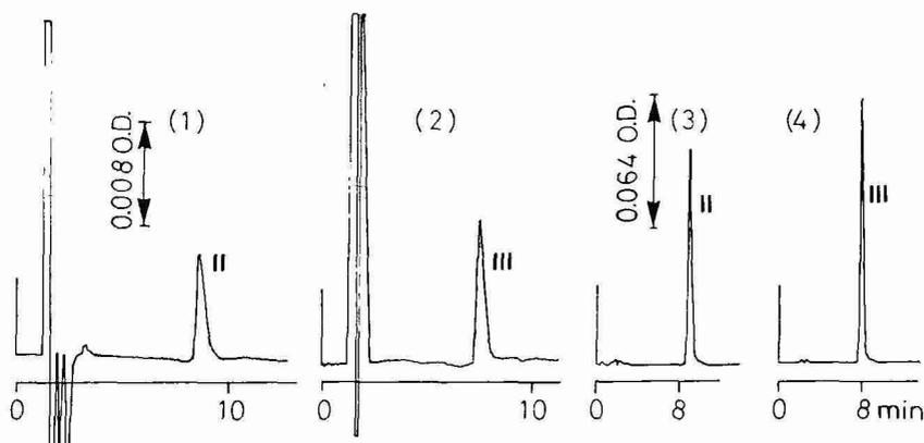
Fig. 5. Comparison of the relative responses to mono- and dialanines with UV and/or post-column detection. Compounds ( $R = C_{12}H_{25}$ ): 1, II,  $40 \mu\text{g}$  ( $143.4 \text{ nmol}$ ), UV at  $210 \text{ nm}$ . 2, III,  $34.92 \mu\text{g}$  ( $93.6 \text{ nmol}$ ), UV at  $210 \text{ nm}$ ; 3, II,  $1 \mu\text{g}$  ( $3.58 \text{ nmol}$ ), post-column detection; 4, III,  $1.74 \mu\text{g}$  ( $4.66 \text{ nmol}$ ), post-column detection.
