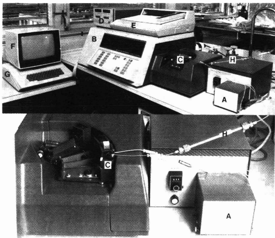
Fig. 1. UV-visible detection set-up used in the HPLC experiments.
