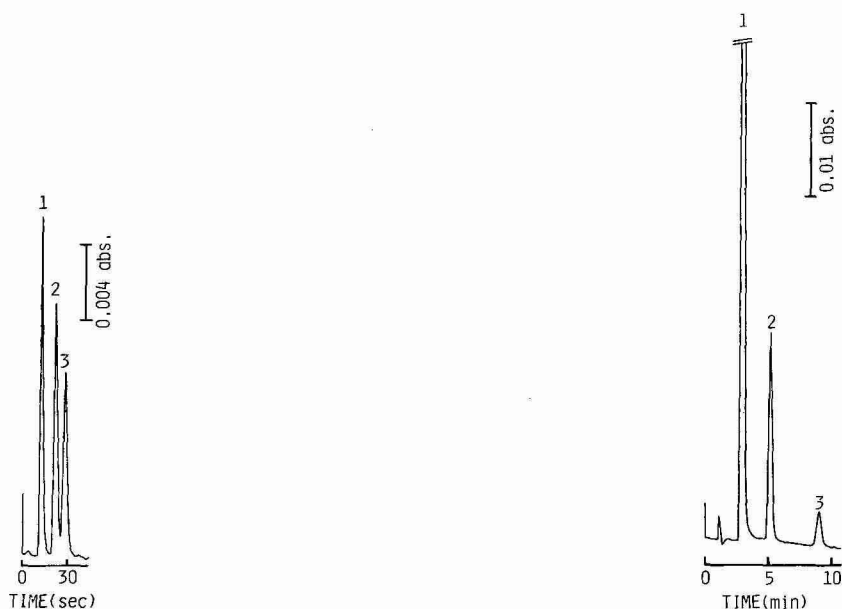
Fig. 3. Rapid separation of an artificial mixture. Column: ODS-Hypersil-3 (3 \mu m), 49 \times 0.3 mm I.D. Mobile phase: methanol–10 mM acetic acid (25:75). Flow-rate: 20 \mu l/min. Peaks: 1 = L-ascorbic acid; 2 = theophylline; 3 = caffeine. Wavelength of UV detection: 265 nm.
