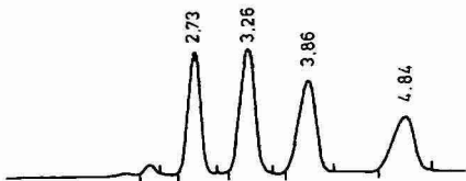
Fig. 2. Separation of dansyl-amino acids: aspartic acid (retention time, t_R = 2.73 min), glycine ( t_R = 3.26 min), arginine ( t_R = 3.86 min) and alanine ( t_R = 4.84 min). Mobile phase: methanol-water (60:40), pH 2.0, flow-rate 1 ml/min. Fluorescence detection: excitation wavelength 360 nm, emission wavelength 470 nm (Biotronik BT 6630).
