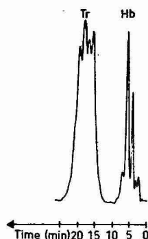
Fig. 1. Elution of focused protein zones by hydrodynamic flow and monitoring by on-tube detection. The sample consisted of 10 \mu\text{g} of human hemoglobin (Hb) and 15 \mu\text{g} of human transferrin (Tr). The experiment was carried out in the HPE equipment 1,2 . The protein zones were recorded as they passed a stationary UV detector monitoring at 280 nm.
