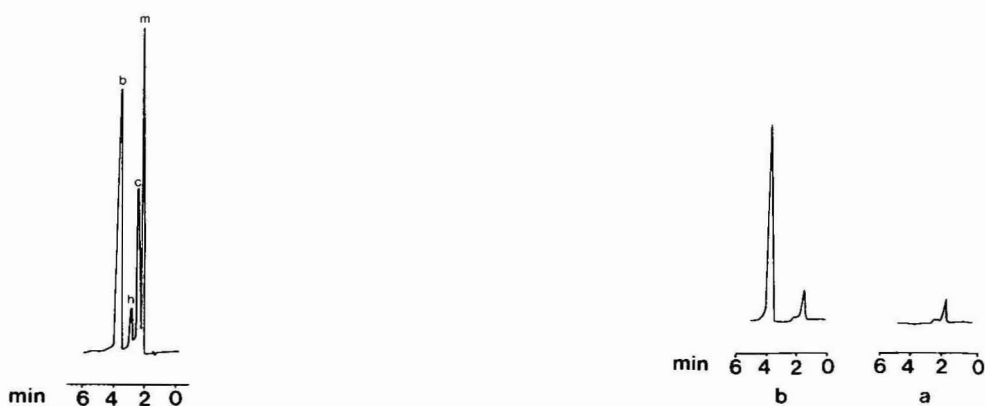
Fig. 1. Separation of commonly used opiates. Peaks: m = morphine; c = codeine; h = heroin; b = buprenorphine.
