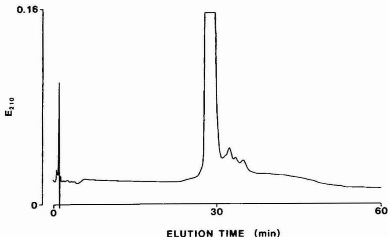
Fig. 9. Separation of 50  $\mu\text{g}$  of crystalline porcine insulin on a 50  $\times$  5.0 mm I.D. PEP-RPC column. Gradient elution, with 0.25 M TEAP (pH 3.0) and 15–35% acetonitrile over 45 min (gradient No. 8), at 1.0 ml/min.
