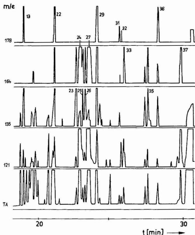
Fig. 2. Mass chromatogram (selected molecular and main fragment ions) of a *tert.*-butylated cresol fraction. The peaks are designated according to Table III (TA = total ionization): 121, main fragment of the *tert.*-butylcresols ( $M-43$ ); 135, main fragment of the *sec.*-butylcresols ( $M-29$ ); 164, molecular ion of the *tert.*-butylcresols; 178, molecular ion of the *sec.*-butylcresols.
