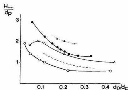
Fig. 5. Dependence of  $\bar{H}_{min}/d_p$  on  $d_p/d_c$ .  $\blacktriangle$ , Chromosorb P with OV-1 ( $d_1 \approx 0.04 \mu\text{m}$ ) (this work);  $\bullet$ , Volaspher A-2 with OV-1 ( $d_1 \approx 0.04 \mu\text{m}$ ) (this work);  $\triangle$ , Chromosorb P without stationary phase<sup>19</sup>.  $\circ$ , glass beads without stationary phase<sup>19</sup>. Broken line, calculated for Volaspher A-2 without stationary phase.
