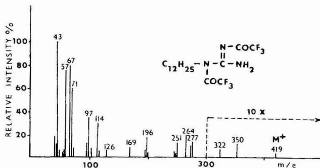
Fig. 2. Mass spectrum of 1-dodecyl-1,2-bis(trifluoroacetyl)guanidine (ionization voltage 70 eV).
