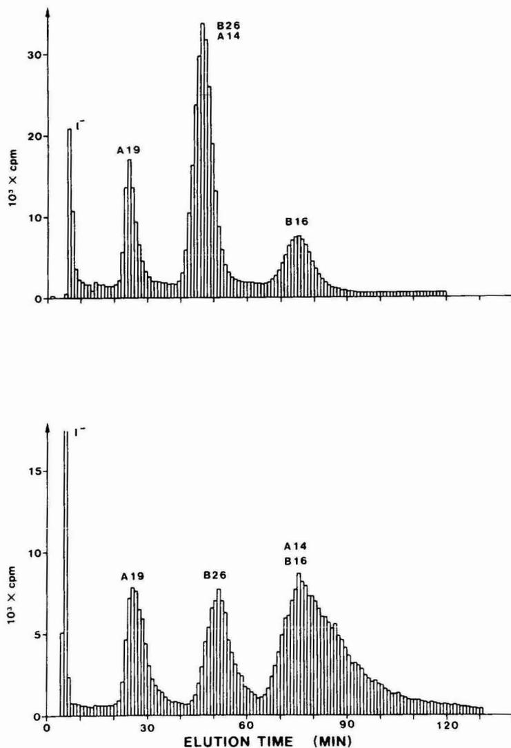
Fig. 12. Isocratic separation of 50  $\mu\text{l}$  of diluted iodination mixture on a 250  $\times$  4.0 mm I.D. column packed with Techogel C<sub>4</sub> (top) or Techogel C<sub>18</sub> (bottom). The columns were eluted with 0.25 M TEAF (pH 6.0)–21.0% isopropanol, at 0.5 ml/min.
