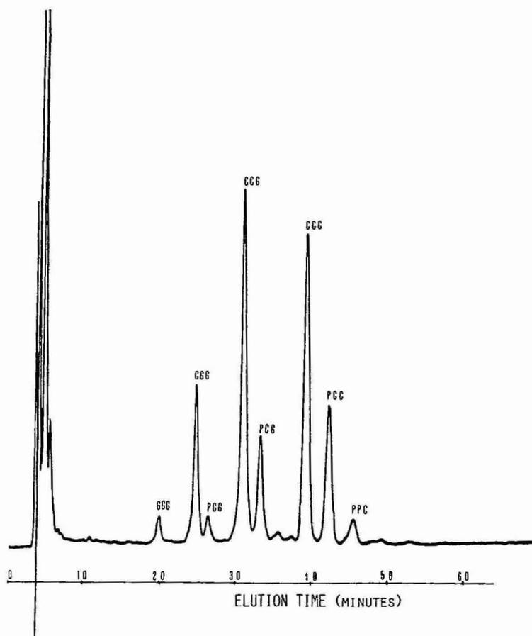
Fig. 1. Separation of triglycerides in *Caloncoba echinata* using two 150 × 4.5 mm I.D. Spherisorb S 3 ODS 2 columns and acetonitrile-tetrahydrofuran (68:32, v/v) as mobile phase at 1.5 ml/min; inlet pressure, 2500 p.s.i. at 20°C; UV detection at 220 nm. Abbreviations: P = palmitic acid; O = oleic acid; H = hydnocarpic acid 16:1 cy; C = chaulmoogric acid 18:1 cy; G = gorlic acid 18:2 cy.
