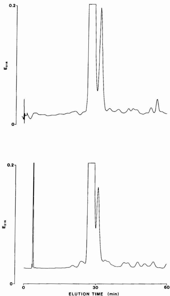
Fig. 8. Separation of 200  $\mu$ g of crystalline porcine insulin on a 250  $\times$  4.6 mm I.D. column packed with Protegil diphenyl (top) or Protegil octyl (bottom). Gradient elution, with 0.25 M TEAP (pH 3.0) and 23–28% acetonitrile (gradient No. 8) over 50 min, at 0.5 ml/min.
