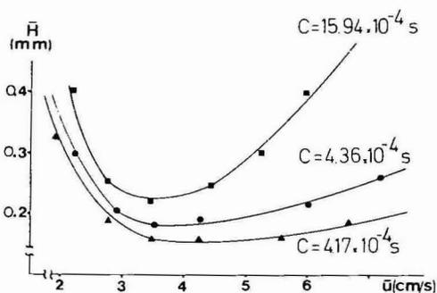
Fig. 4. Plot of  $\bar{H}$  versus average linear gas velocity for the columns in Table II.  $\blacksquare$ , 0.8;  $\bullet$ , 0.6;  $\blacktriangle$ , 0.5 mm I.D. The  $C$  terms in eqn. 2 are shown.
