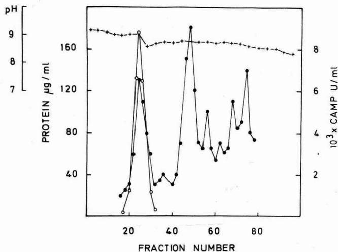
Fig. 3. Chromatofocusing of the CAMP-factor on polybuffer exchanger PBE 94 (column,  $40 \times 1$  cm I.D.). Separation of CAMP-factor (fraction Nos. 18–32) from contaminating material (fraction Nos. 40–53) was done by elution with polybuffer 96–hydrochloric acid at pH 7.0. Starting buffer, 0.025 M ethanolamine–hydrochloric acid (pH 9.4); flow-rate, 12 ml/h. Protein  $\mu$ g/ml (—●—●—); activity of CAMP-factor U/ml (—○—○—).
