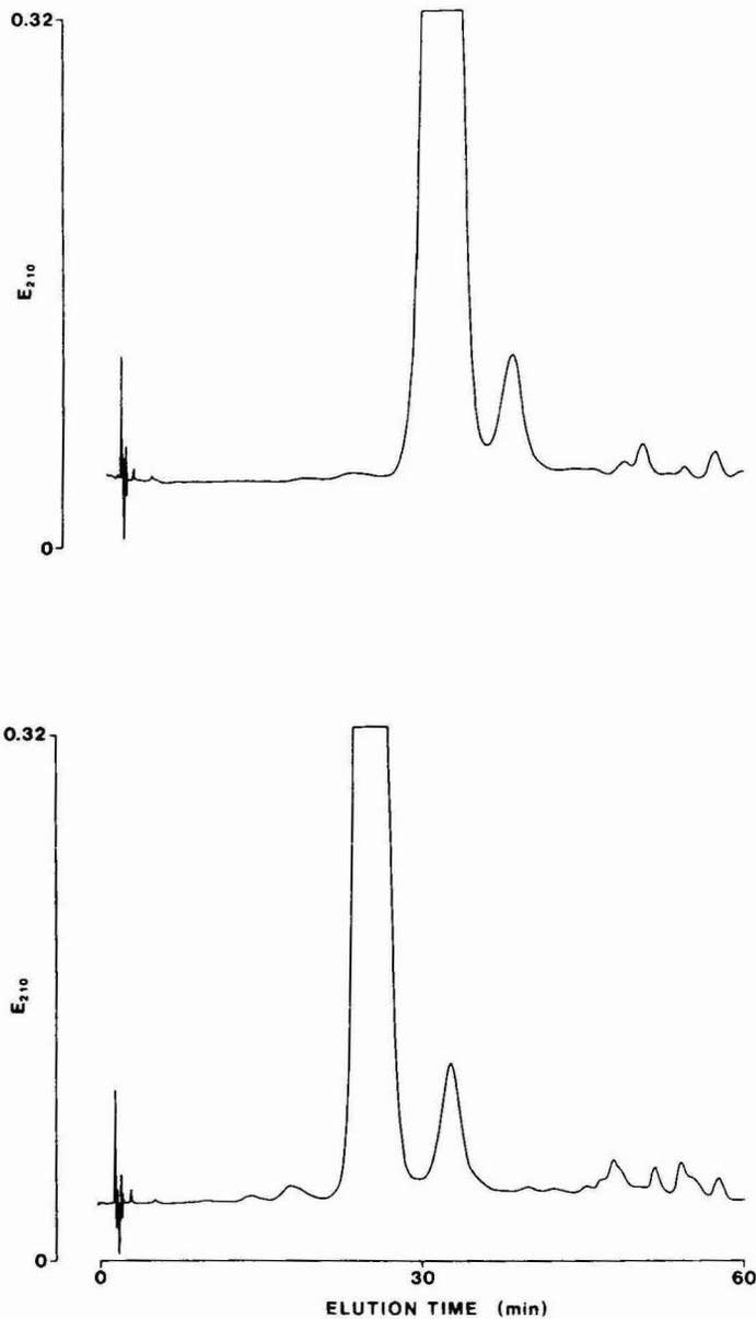
Fig. 10. Separation of 200  $\mu\text{g}$  of crystalline porcine insulin on a  $150 \times 4.0$  mm I.D. column packed with PRP-1 (top) or PLRP-S (bottom). Gradient elution, with 0.25 M TEAP (pH 3.0) and 22–25.5% acetonitrile (gradient No. 8), at 1.0 ml/min.
