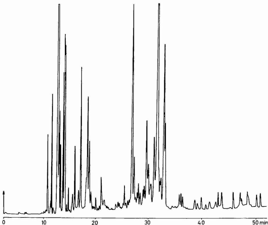
Fig. 6. Chromatogram of extract of *Santolina rosmarinifolia* obtained on a 4% SE-30 on Volaspher A-2 (120–140-mesh) column (5.5 m × 1.0 mm I.D.). Carrier gas, H<sub>2</sub> (8 cm/s). Temperature, programmed from 40°C at 5°C/min to 200°C.
