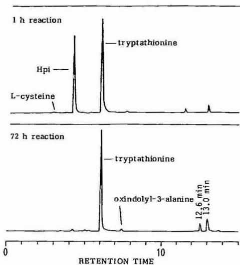
Fig. 1. HPLC trace of samples taken from the tryptathionine reaction mixture after 1 h and 72 h at 289 nm. L-Cysteine does not absorb maximally at this wavelength.
