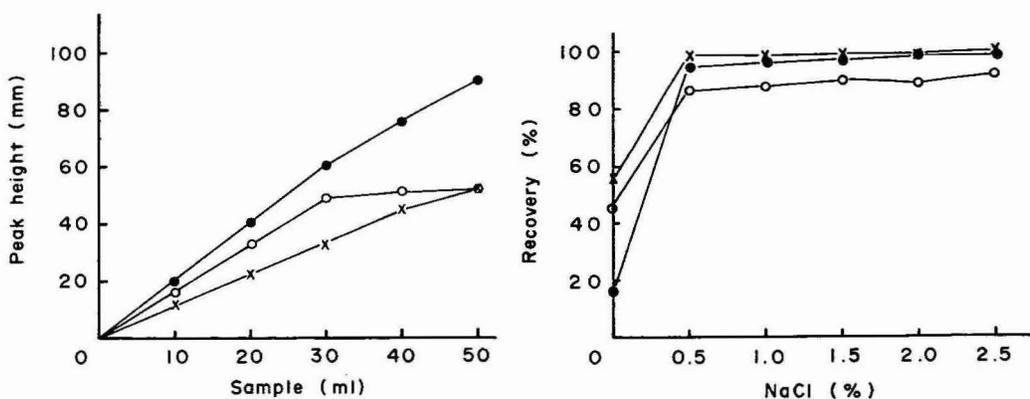
Fig. 7. Relationship between the volume of the sample poured into the Sep-Pak C<sub>18</sub> cartridge and the peak height.
