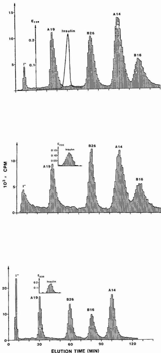
Fig. 11. Isocratic separation of 50  $\mu$ l of diluted iodination mixture on a 250  $\times$  4.6 mm I.D. TSK ODS-120T column (bottom), a 150  $\times$  4.0 mm I.D. Spherisorb ODS2 column (middle) or a LiChrosorb RP-18 column (250  $\times$  4.0 mm I.D.) (top), with 0.25 M TEAF (pH 6.0)-isopropanol concentrations of 21.5, 21.5 and 20.5% (from top to bottom). Flow-rate, 0.5 ml/min.
