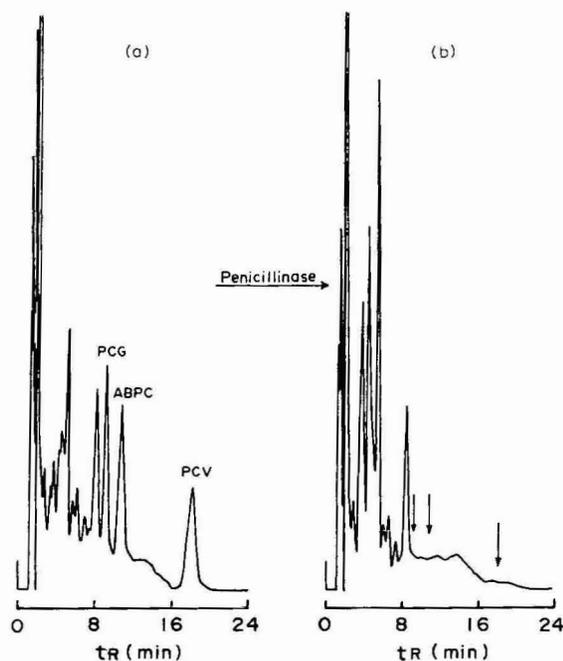
Fig. 12. Liquid chromatograms obtained from a milk sample by the overall procedure (a) and the sample solution treated with penicillinase (b). Sample spiked with 0.5  $\mu\text{g/g}$  each of sodium PCG, potassium PCV and ABPC. Operating conditions as in Fig. 6.
