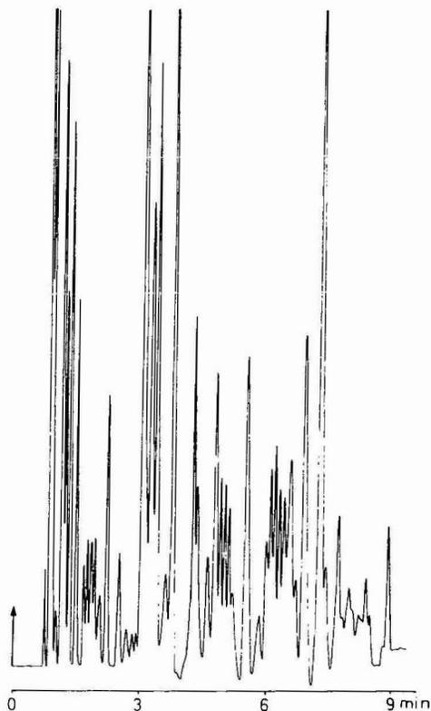
Fig. 7. Chromatogram for direct injection of naphtha into a 4% OV-1 on 120–140-mesh Volaspher A-2 column (3 m  $\times$  0.5 mm I.D.). Carrier gas,  $N_2$  (4.5 cm/s). Temperature, programmed from 60°C at 10°C/min to 210°C.
