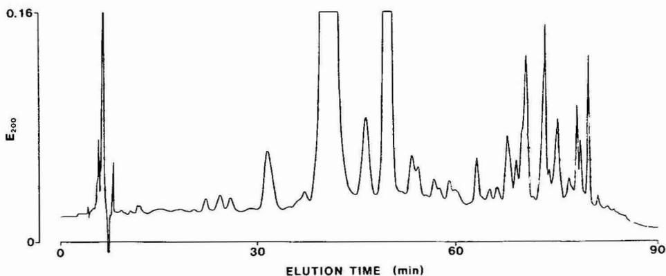
Fig. 5. Separation of 100  $\mu\text{g}$  of crystalline porcine insulin on a 250  $\times$  4.6 mm I.D. TSK ODS-120T column. Gradient elution, with 0.25 *M* TEAP (pH 3.0) and 27.5–32.5% acetonitrile over 70 min (gradient No. 8) at 0.5 ml/min.
