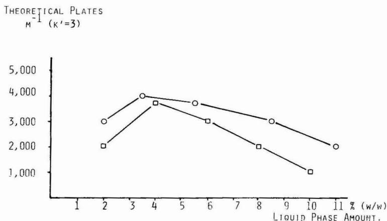
Fig. 1. Dependence of specific efficiency on liquid loading.  $d_c = 1.0$  mm;  $L = 2$  m;  $d_p = 0.113$  mm; carrier gas,  $\text{N}_2$ . ○, non-polar phase (SE-30); □, polar phase (Carbowax 20M).
