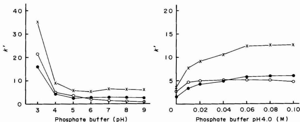
Fig. 3. Effect of the pH of the phosphate buffer added to the mobile phase on the  $k'$  of PCG, PCV and ABPC. Mobile phase, methanol-water- $0.2 \text{ M}$  phosphate buffer (pH 3.0–9.0) (5:13:2) containing  $10 \text{ mM}$  sodium 1-heptanesulphonate. Other conditions as in Fig. 1.
