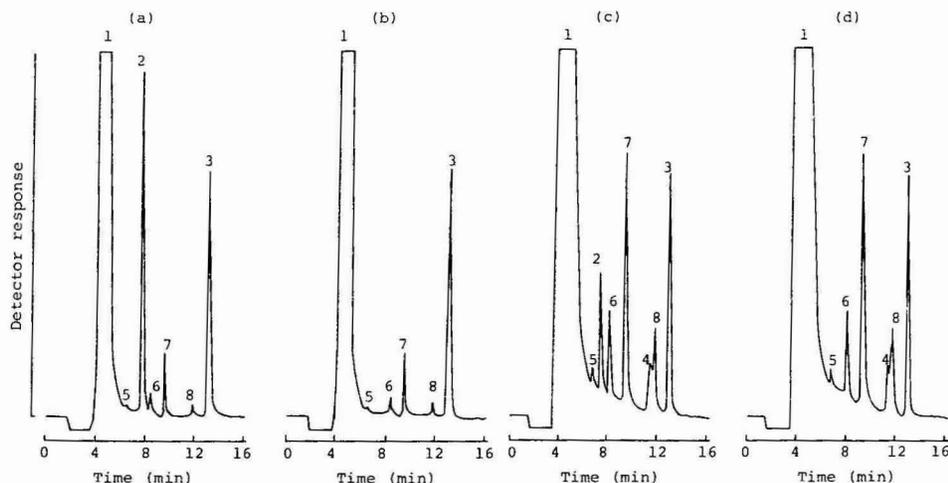
Fig. 1. Chromatograms obtained with the enzyme preparations from (a) adrenal medulla, (c) brain and (b) and (d) their blanks, respectively. Portions ( $100\ \mu\text{l}$ ) of the enzyme preparations were treated according to the procedure. Peaks: 1 = norepinephrine; 2 = epinephrine; 3 = isoproterenol; 4 = dopamine (endogenous); 5–8 = impurities in commercial norepinephrine. PNMT activity (pmol/min/mg protein): (a) 230; (c) 0.52. Detector sensitivity: (a) and (b) 2; (c) and (d) 8.
