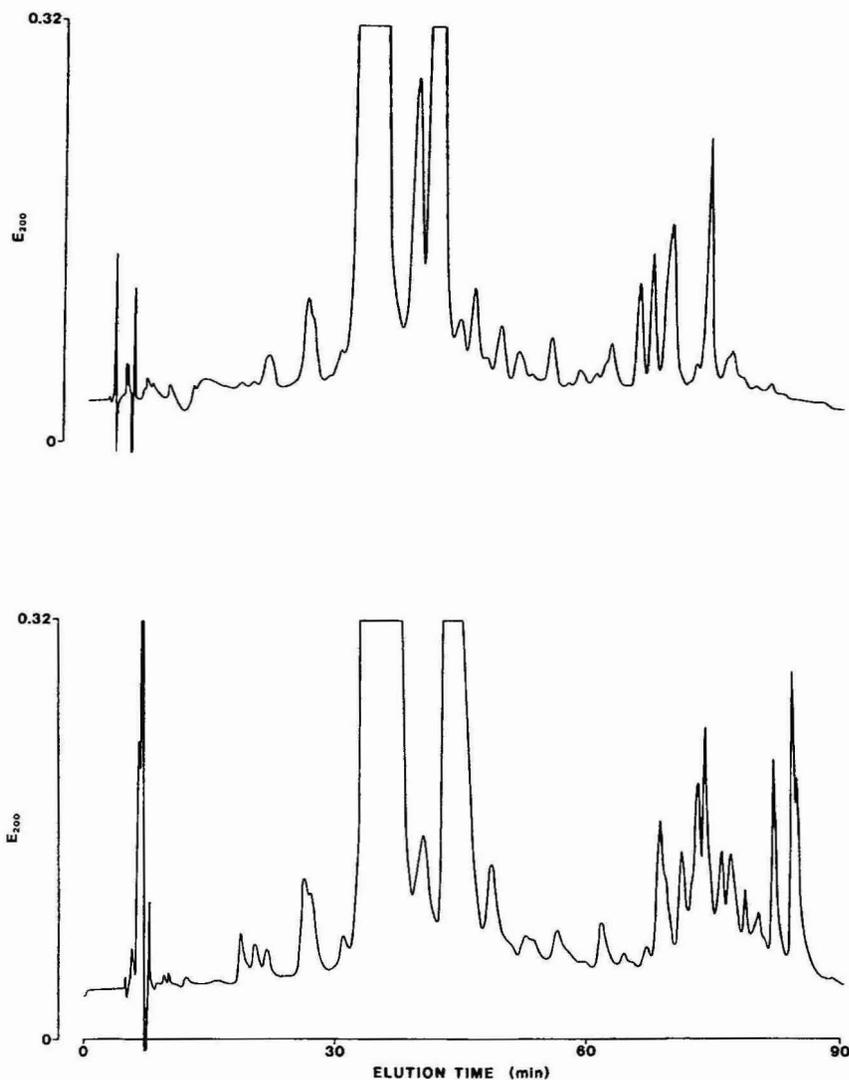
Fig. 7. Separation of 200  $\mu\text{g}$  of crystalline porcine insulin on a 250  $\times$  4.0 mm I.D. Techogel C<sub>4</sub> column (top) or a 250  $\times$  4.0 mm I.D. Techogel C<sub>18</sub> column (bottom). Gradient elution, with 0.25 M TEAP (pH 3.0) and 25–27.5% acetonitrile (gradient No. 8) for 60 min, at 0.5 ml/min.
