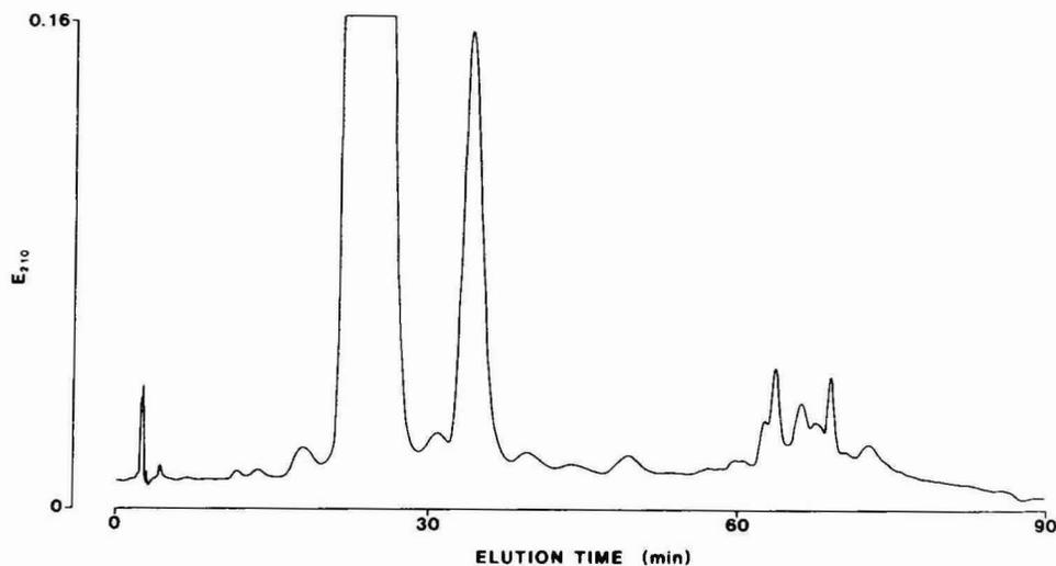
Fig. 6. Separation of 200  $\mu\text{g}$  of crystalline porcine insulin on a  $150 \times 3.9$  mm I.D. Nova-Pak  $\text{C}_{18}$  column. Gradient elution, with 0.25 M TEAP (pH 3.0) and 23.5–29% acetonitrile (gradient No. 8) for 60 min, at 0.5 ml/min.
