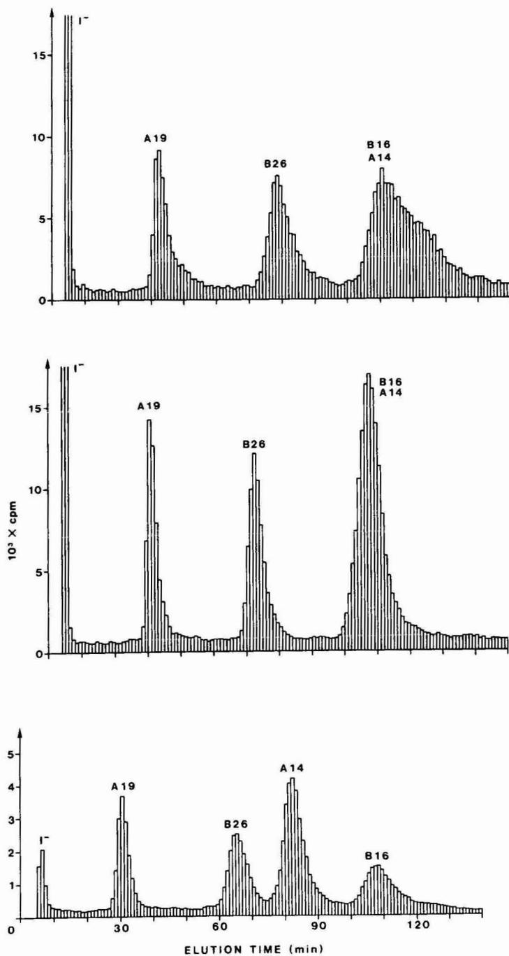
Fig. 14. Isocratic separation of 50  $\mu$ l of diluted iodination mixture on three different LiChrosorb RP-18 columns (250  $\times$  4.0 mm I.D.) eluted with 0.25 M TEAF (pH 6.0) containing (from top to bottom) 22.0, 21.0 and 21.0% isopropanol. Flow-rate 0.5 ml/min.
