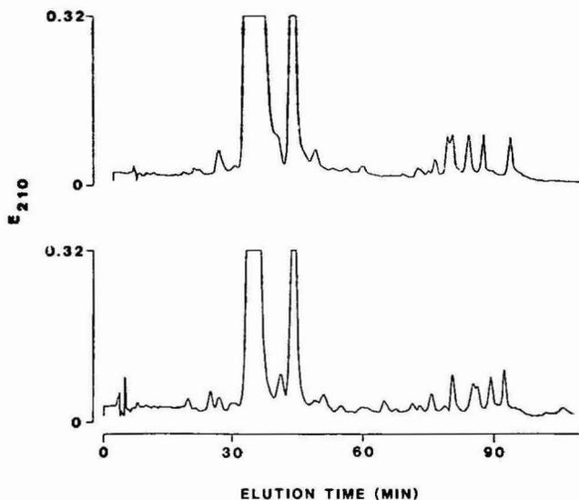
Fig. 4. Separation of 200  $\mu\text{g}$  of crystalline porcine insulin on a 250  $\times$  8.0 mm I.D. Vydac 218 TPB 5 column (top), or a 250  $\times$  4.0 mm I.D. Spherisorb ODS2 column (bottom). Gradient elution, with 0.25 *M* TEAP (pH 3.0) and 23–28% acetonitrile over 60 min (gradient No. 8). Flow-rate, 1.0 ml/min (top), 0.5 ml/min (bottom).
