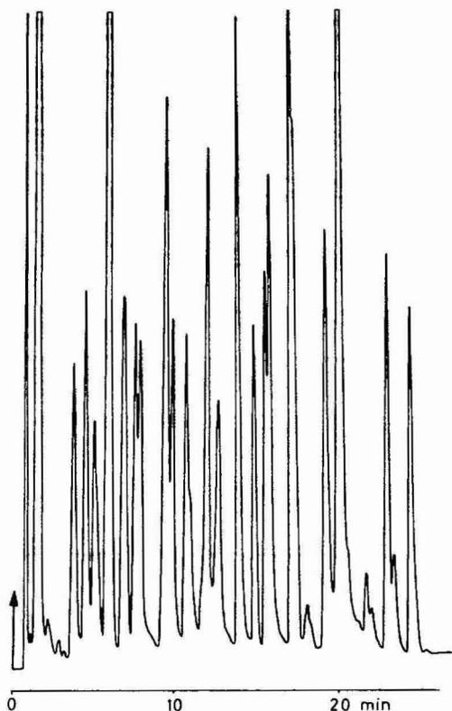
Fig. 8. Chromatogram of an organic extract of a wine obtained on a 5% OV-275 on Volaspher A-2 (120-140-mesh) column (2 m  $\times$  1 mm I.D.). Carrier gas, N<sub>2</sub> (4 cm/s). Temperature, programmed from 70°C at 5°C/min to 200°C.
