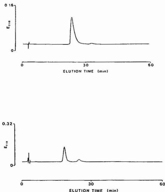
Fig. 1. Isocratic separation of  $5 \mu\text{g}$  of crystalline porcine insulin on a  $250 \times 4.0 \text{ mm}$  I.D. LiChrosorb RP-18 column eluted with 0.1% TFA–27.0% acetonitrile (upper curve) and 0.25 M TEAP–22.0% acetonitrile (lower curve), at 0.5 ml/min.
