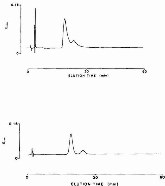
Fig. 2. Isocratic separation of 5  $\mu\text{g}$  of crystalline porcine insulin on a  $100 \times 3.0$  mm I.D. glass cartridge packed with Chrompack  $\text{C}_{18}$ . Elution was performed at 0.5 ml/min, with 0.1% TFA-23.5% acetonitrile (upper curve) and 0.25 M TEAP-22.5% acetonitrile (lower curve).
