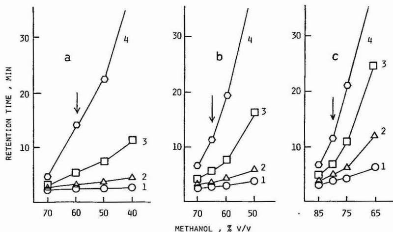
Fig. 1. Effect of methanol content in the eluent methanol-1/15 *M* phosphate buffer (pH 6.8) on the retention of  $R_2NCS_2Na$  on  $C_{18}$ -bonded silica in the presence of (a) TMAB, (b) TBAB and (c) CTAB. Carbamates: 1 =  $Me_2NCS_2Na$ ; 2 =  $Et_2NCS_2Na$ ; 3 =  $Pr_2NCS_2Na$ ; 4 =  $Bu_2NCS_2Na$ .
