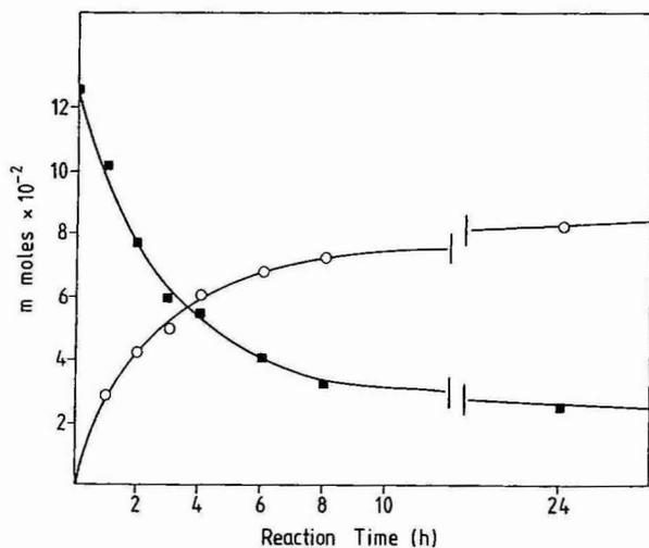
Fig. 2. The formation of tryptathionine (O) and the consumption of Hpi (■) plotted against time of reaction.
