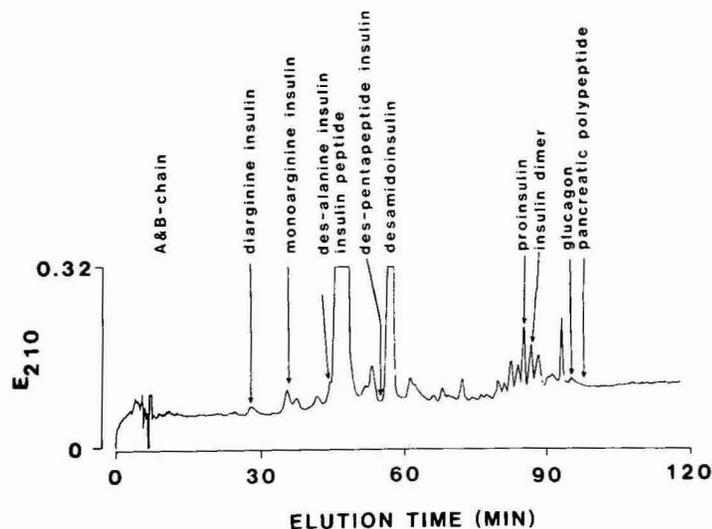
Fig. 3. Separation of 200  $\mu\text{g}$  of crystalline porcine insulin on a  $250 \times 4.0$  mm I.D. LiChrosorb RP-18 column. Gradient elution, with 0.25 M TEAP (pH 3.0) and 23-28% acetonitrile over 60 min (gradient No. 8), at 0.5 ml/min.
