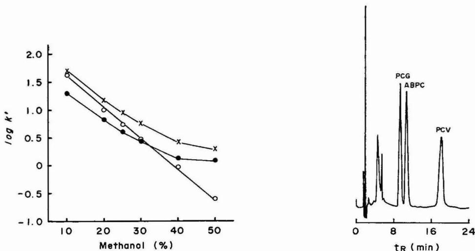
Fig. 5. Effect of the concentration of methanol on the  $k'$  of PCG, PCV and ABPC. Mobile phase, methanol-water containing 0.02 *M* phosphate buffer (pH 4.0) and 10 *mM* sodium 1-heptanesulphonate. Other conditions as in Fig. 1.
