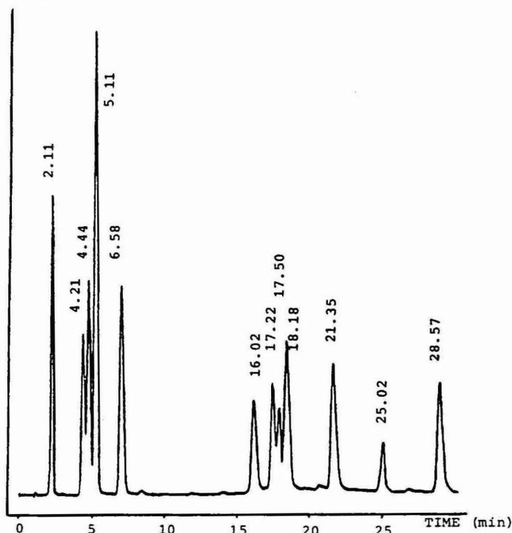
Fig. 1. The retention times of caffeoylquinic acid derivatives and flavonoids eluted using the linear gradient on a Spherisorb  $C_{18}$  column. A list of the compounds separated is given in Table I. For the elution system see Experimental.
