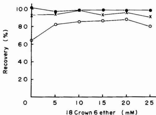
Fig. 9. Effect of 18-crown-6 ether concentration in the rinsing solution [containing 2% (w/v) sodium chloride and 10% (v/v) methanol] for the Sep-Pak  $C_{18}$  cartridge on the recoveries of PCG, PCV and ABPC.
