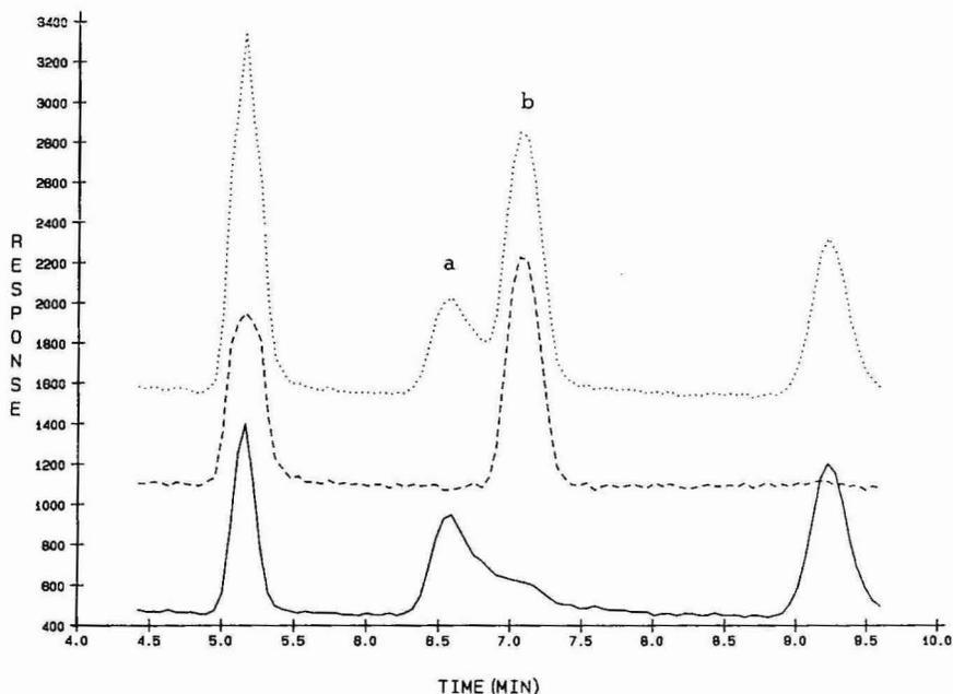
Fig. 2. Chromatograms which illustrate voltage resolution. Response at 900 mV potential (.....), response at 750 mV (—), difference chromatogram (upper trace—lower trace) (-----). a = 0.47 nmol of 2,3-dihydroxybenzoic acid, b = 13 nmol of 3,5-dihydroxybenzoic acid.
