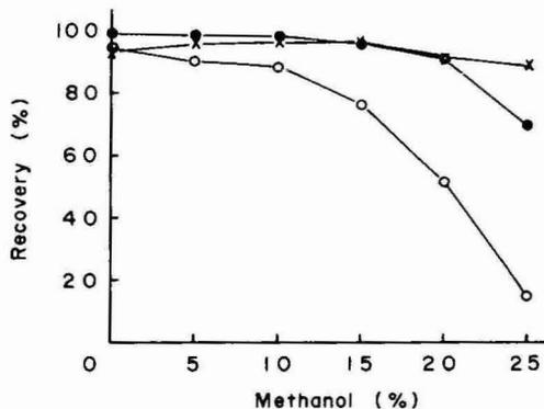
Fig. 10. Effect of methanol concentration in the rinsing solution [containing 20 mM 18-crown-6 ether and 2% (w/v) sodium chloride] for the Sep-Pak  $C_{18}$  cartridge on the recoveries of PCG, PCV and ABPC.
