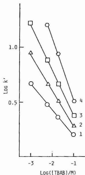
Fig. 7. Variation of log capacity factor ( $k'$ ) with log concentration of TBAB. Numbers as in Fig. 1.
